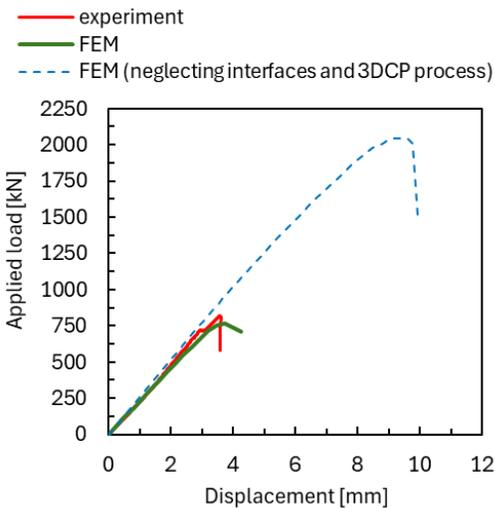
**Fig. 4 Comparison of experimental and numerical load-displacement diagrams for the analyses with and without the consideration of the imperfections and weak layer interfaces**
