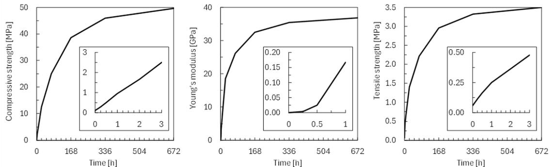
**Fig. 2** Time dependent evolution of main material parameters  $f_c$ ,  $E$ ,  $f_t$ .
