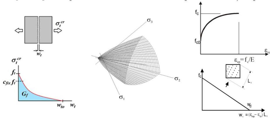
**Fig. 1** Main features of the used fracture-plastic material model
