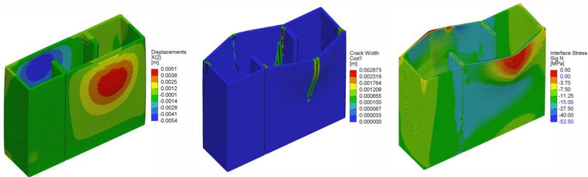
**Fig. 3 Simulation and failure mechanism of 3D printed concrete wall during compression test.**
