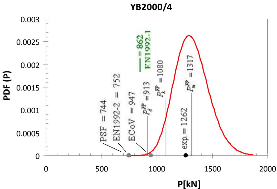
Figure 7. Comparison of safety margins for Beam YB2000/4.
