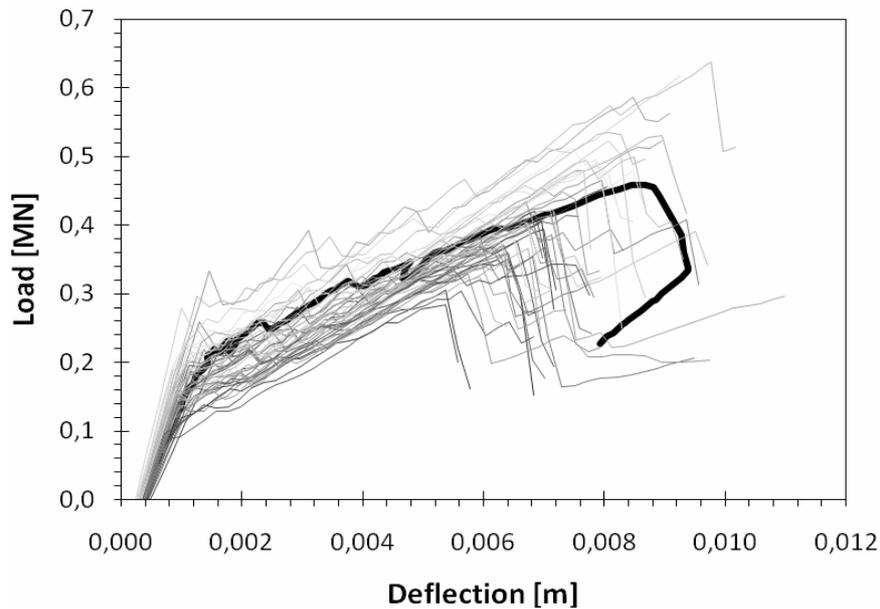
Figure 4. Beam YB2000/0. Load-displacement diagrams of 50 simulations and experiment.
