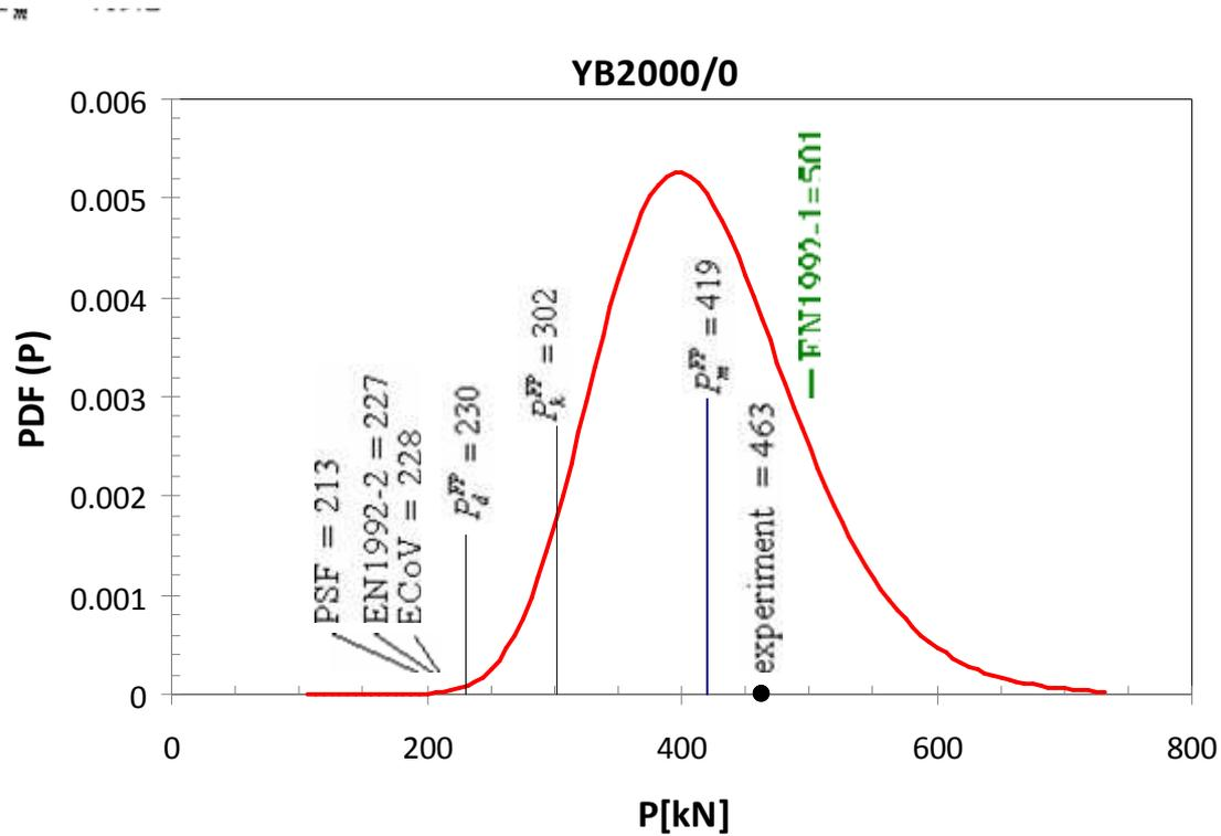
Figure 6. Comparison of safety margins for Beam YB2000/0.
