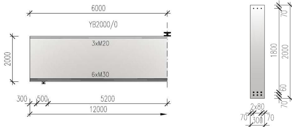
Figure 1 Beam YB2000/0 dimensions and reinforcement.
