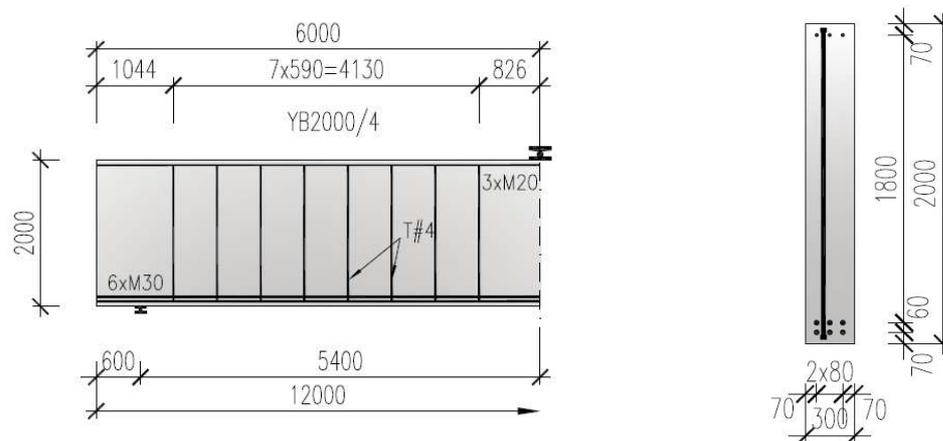
Figure 2. Beam YB2000/4 dimensions and reinforcement.
