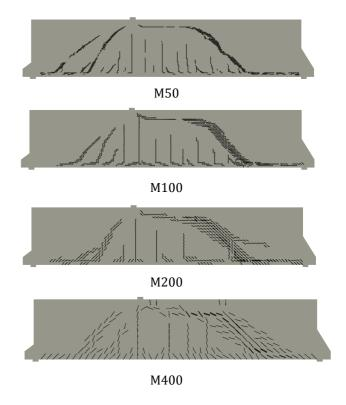
Figure 9: Crack patterns for low order meshes.
