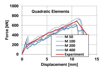
Figure 8: Mesh size effect for quadratic elements.
