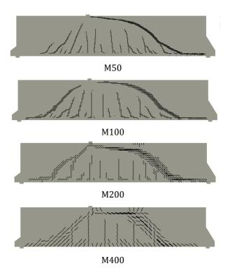
Figure 10: Crack patterns for quadratic meshes.
