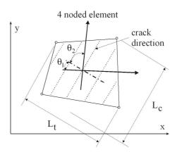
Figure 3: Crack band formulation.
