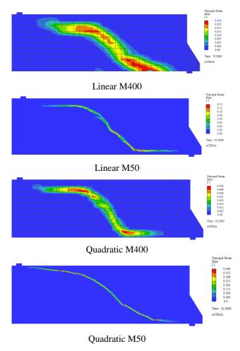
Figure 11: Strain localization.
