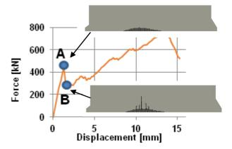
Figure 12: Strain localization at the crack initiation.
