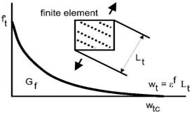
Figure 2: Crack opening law according to Hordijk [8].
