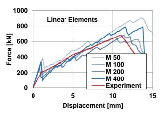
Figure 7: Mesh size effect for low order elements.
