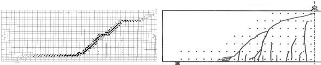
Fig. 3 Numerical and experimental crack pattern.
