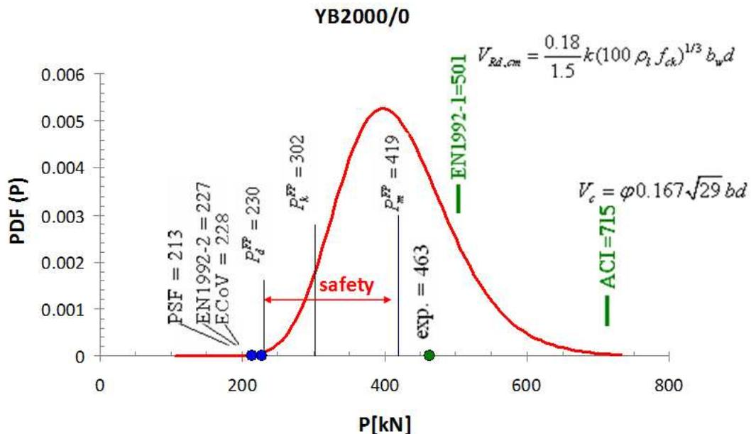
Fig. 4 Design resistance of large beam by Yoshida [8] according to various safety formats and codes.
