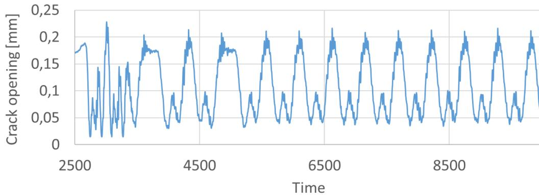
**Fig. 16:** Prediction of bridge maximum crack openings by Digital Twin model during train overpass.
