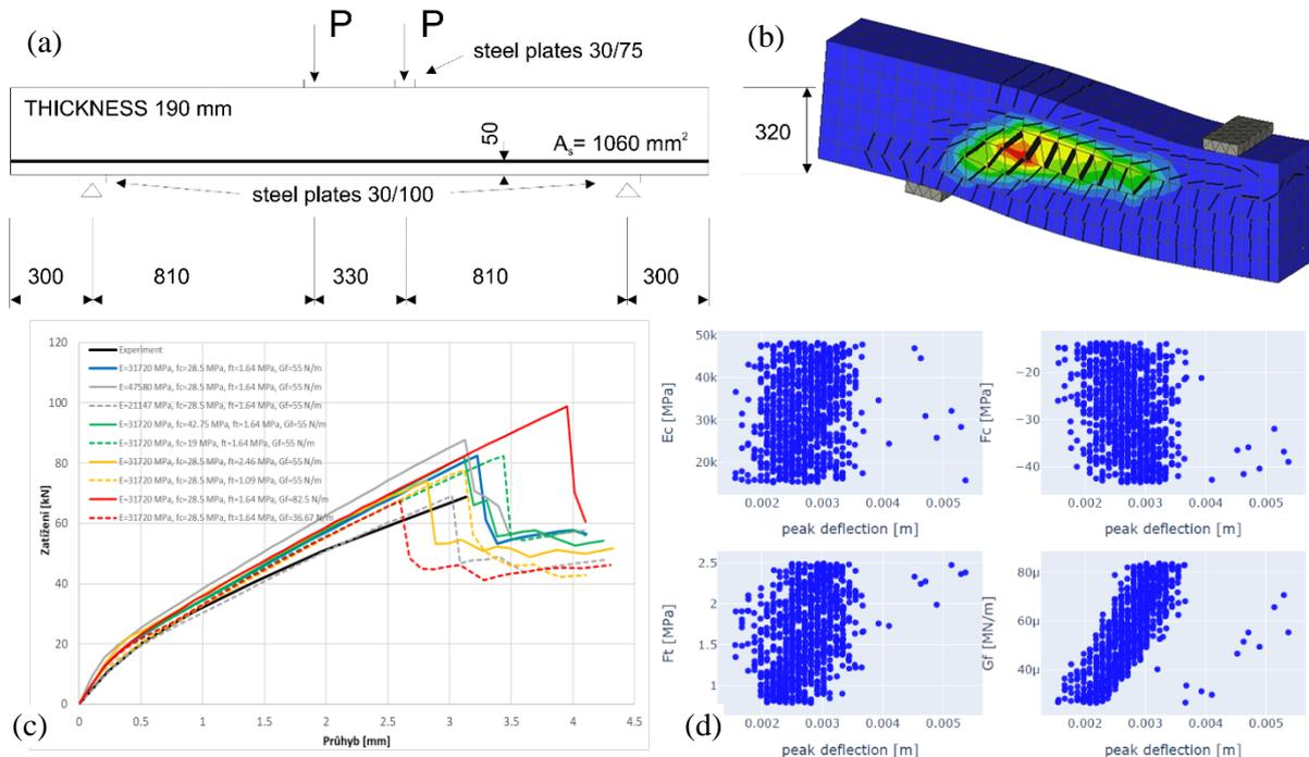
**Fig. 3.** Shear beam test example [5] used for the evaluation of ANN accuracy for the model parameter identification. (a) geometry, (b) numerical model failure simulation, (c) load-displacement diagrams, (d) distribution of the main parameters in the dataset of 1000 training and testing samples.
