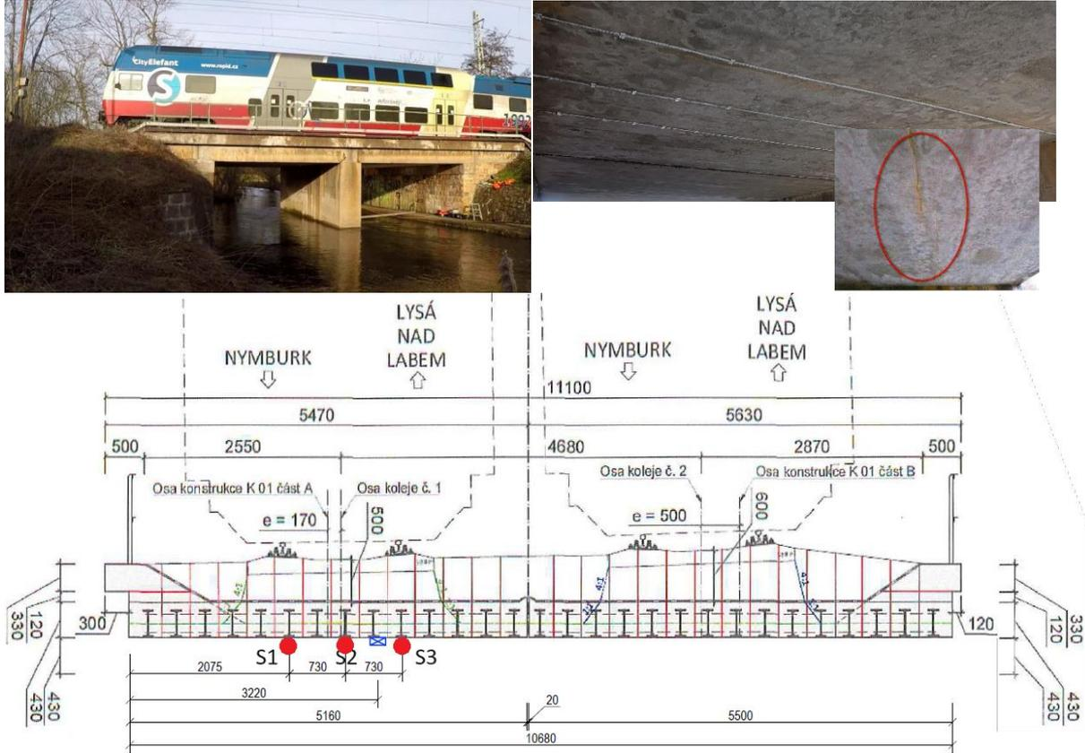
**Fig. 9.** Pilot bridge application example, small railway bridge at Kostomlaty, Czech Republic with the sensor location S1, S2 and S3.
