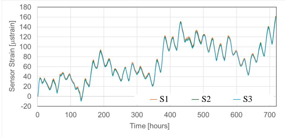
**Fig. 11.** Simulation of the sensor strains evolution due to measured ambient temperatures.
