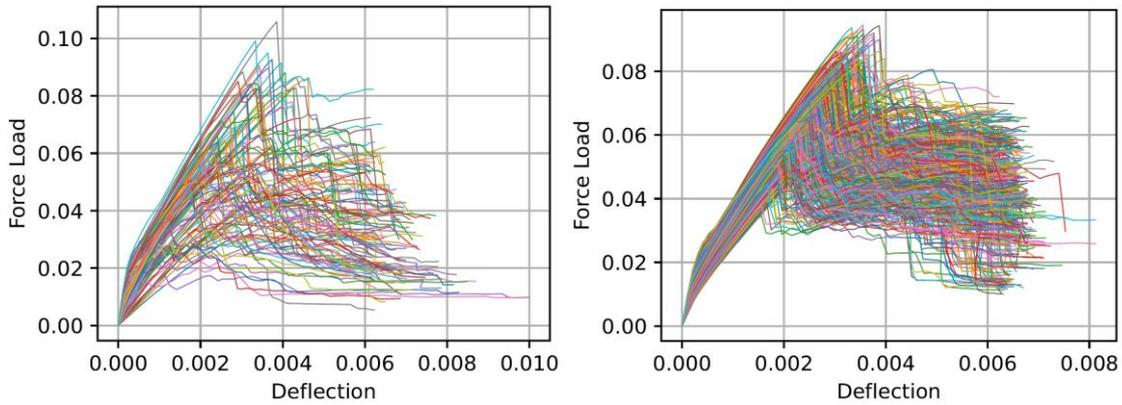
Fig. 7. Simulation data for ANN surrogate model training and testing (left) dataset A with 100 samples, (right) dataset B with 400 samples.
