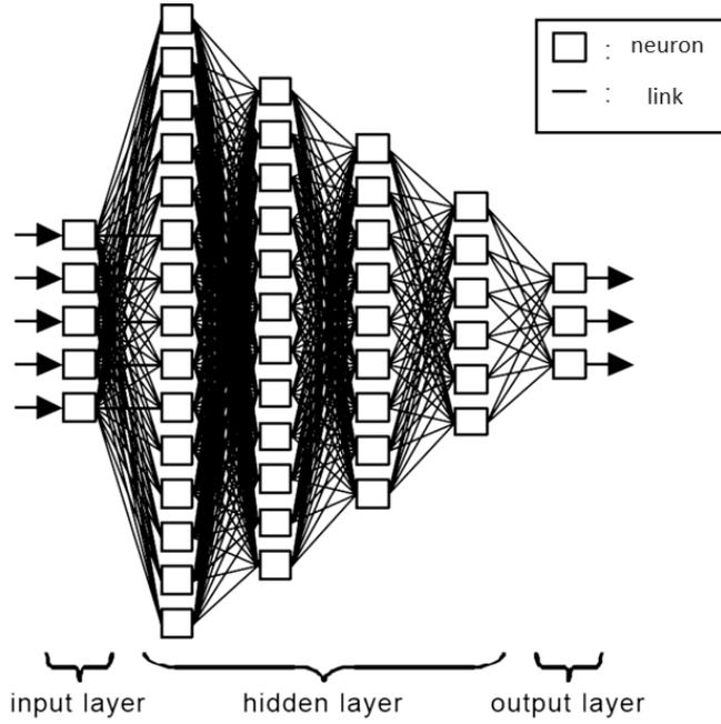
Fig. 6. Dense NN model with 4 hidden layers: 1000, 5000, 500 and 500 neurons in each layer fully connected.
