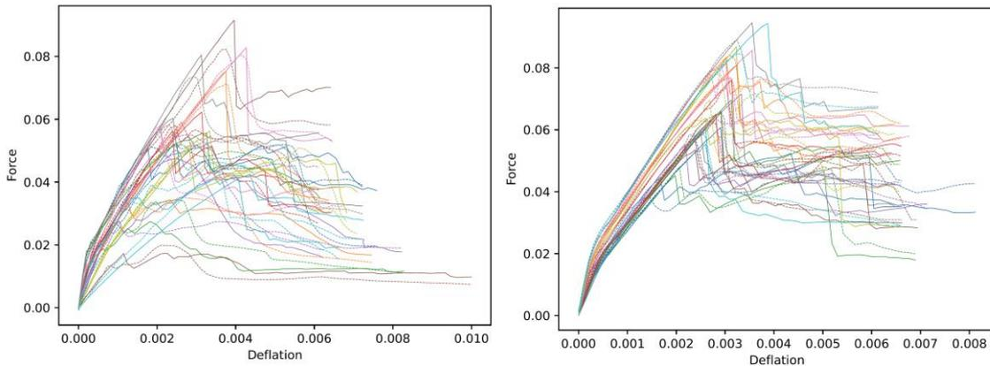
Fig. 8. Accuracy of ANN surrogate model in predicting the response of the testing shear beam structure, (left) dataset A, (right) dataset B, solid lines indicate the response from FE simulation, dotted lines indicate the prediction by the surrogate Dense-NN model.
