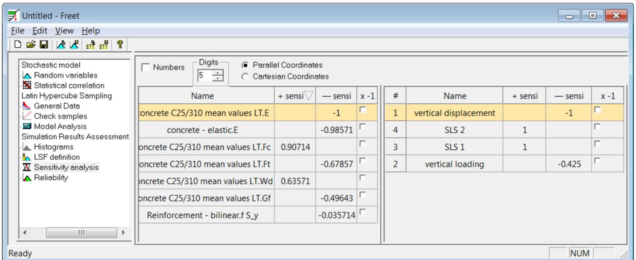
Figure 95 Comparison of quotients from the correlation matrix with sensitivity of vertical displacement.
