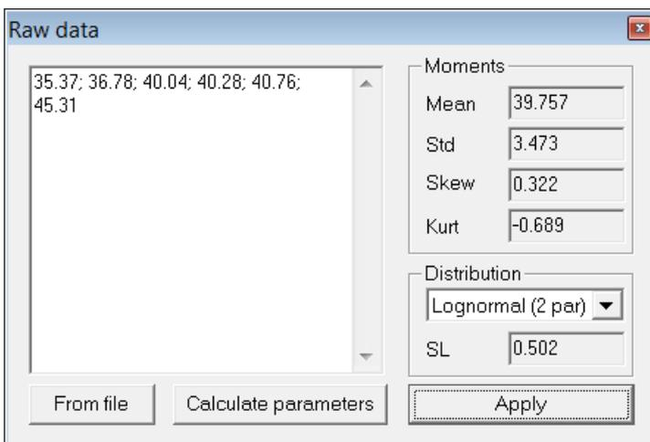
Figure 70 Determination of a type of distribution and its parameters from raw data
