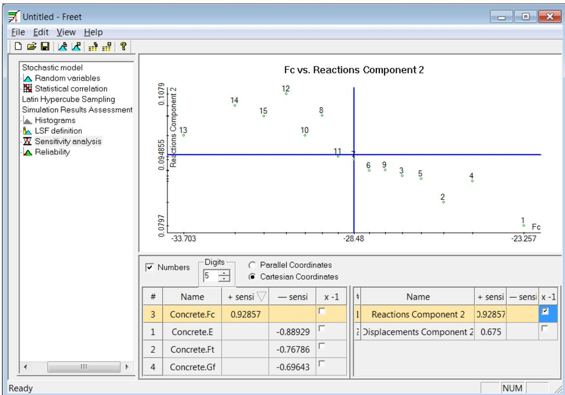
Figure 29 FREET – Sensitivity analysis of Reaction component 2 on compressive strength fc (Cartesian coordinates)
