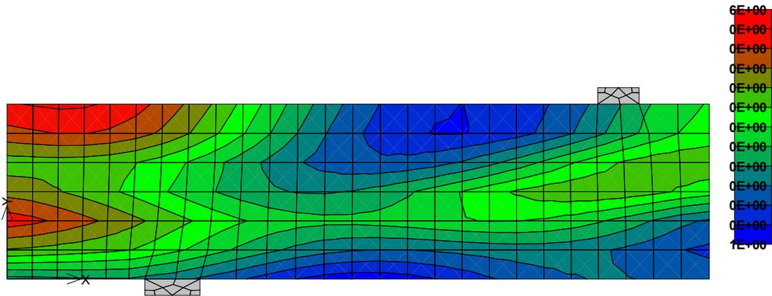
**Figure 57 ATENA postprocessor – demonstration of different correlation lengths in horizontal and vertical direction**
