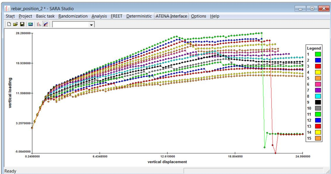
Figure 78 LD diagrams of 15 variants and additional rebars (10Ø8 in total)
