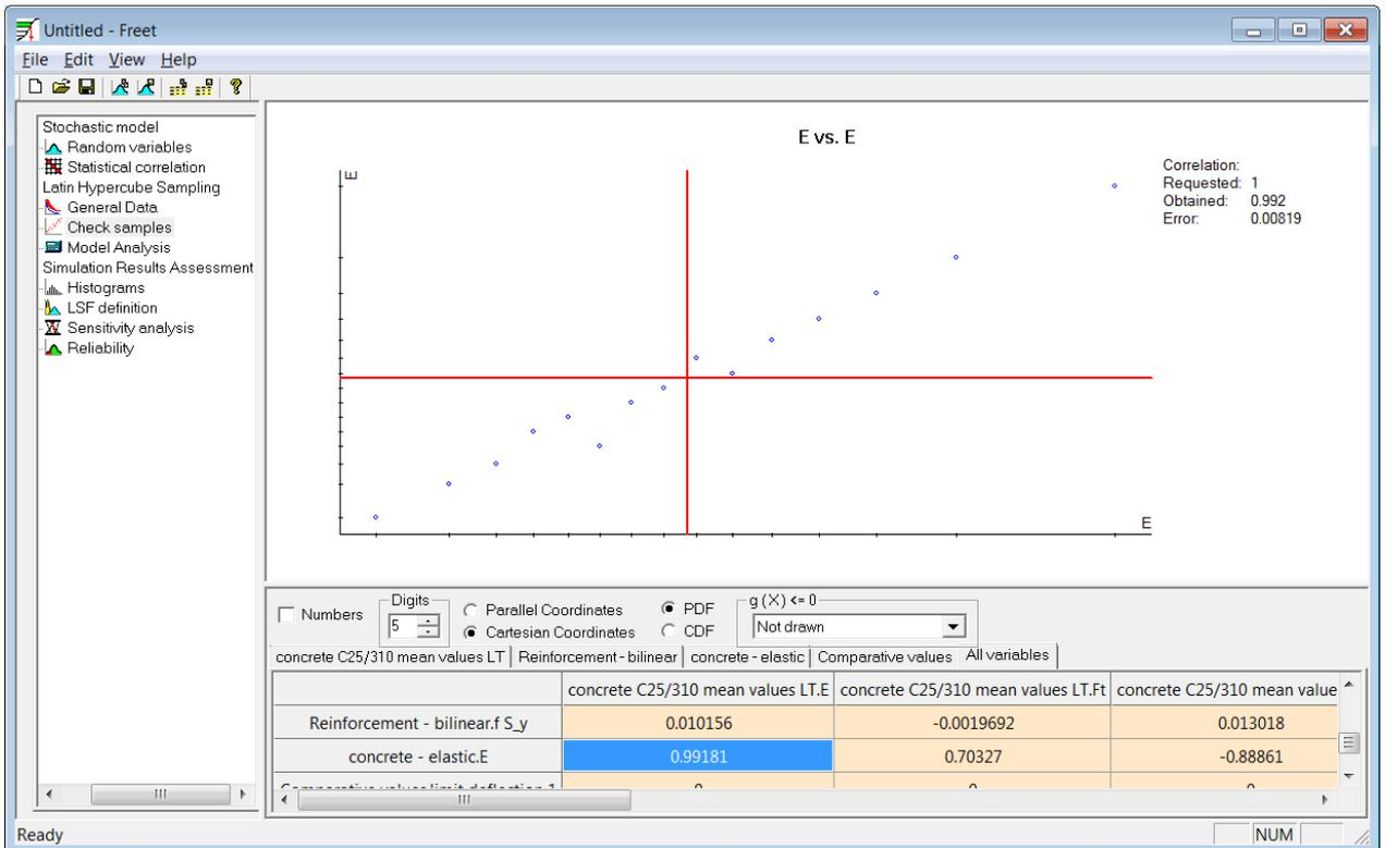
Figure 94 Obtained correlation between elastic moduli of concrete.
