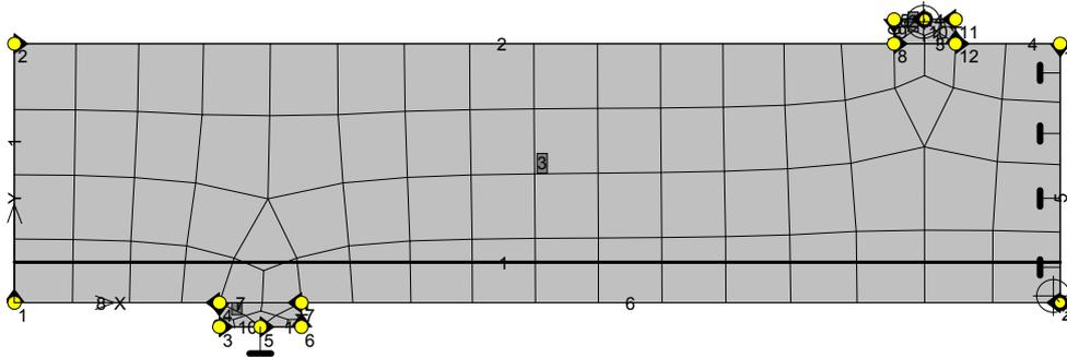
**Figure 2** FE mesh, monitoring points and boundary conditions.
