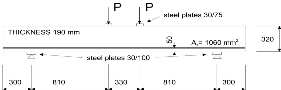
Figure 1 Geometry and loading of Leonhard's beam
