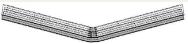
Stress in reinforcement due to large deflection
