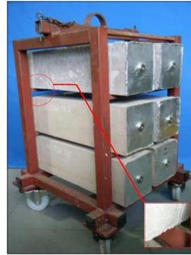
**Figure 77: Scheme of specimen for free shrinkage measurements (left), beams during the test (right) [21]**
