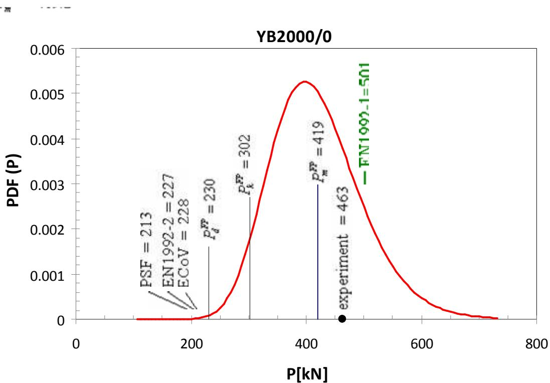
Figure 6. Comparison of safety margins for Beam YB2000/0.
