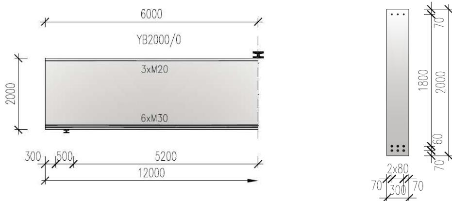
Figure 1 Beam YB2000/0 dimensions and reinforcement.
