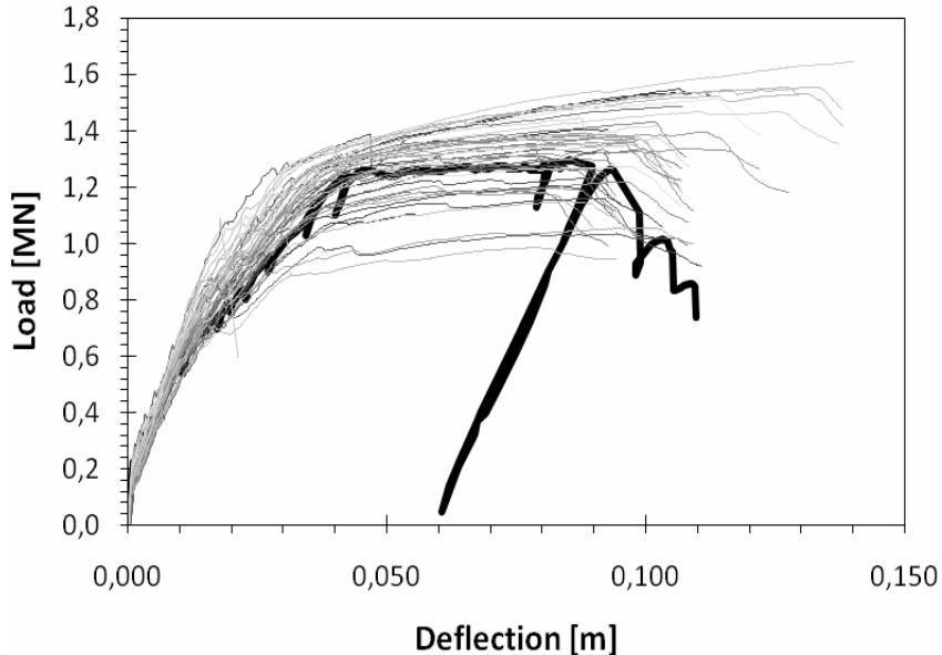
Figure 5. Beam YB2000/4. Load-displacement diagrams of 50 simulations and experiment.
