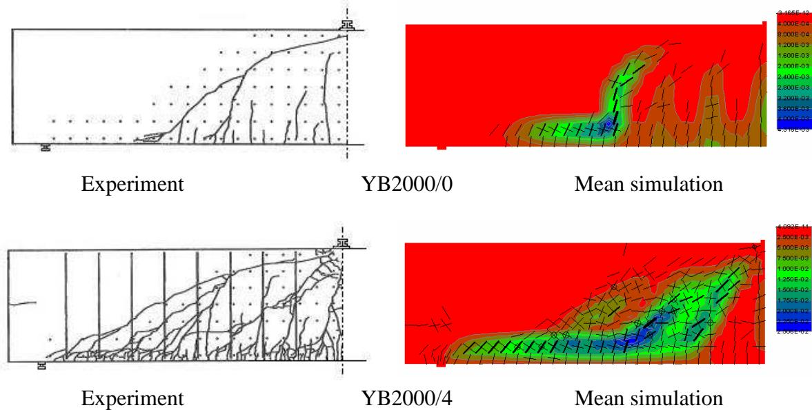
Fig.8 Failure modes. Analysis: cracks and iso-lines of fracture strains indicating damage.
