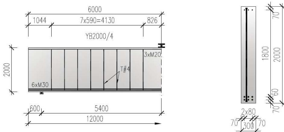
Figure 2. Beam YB2000/4 dimensions and reinforcement.
