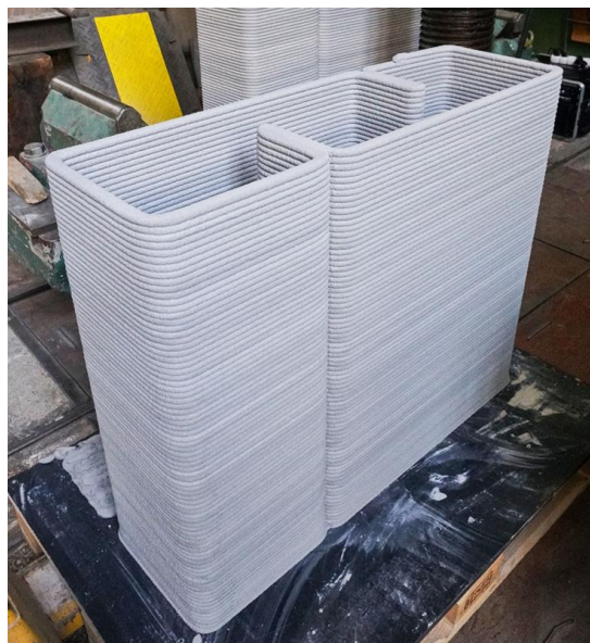
Fig. 1 Photo of the 3D-printed wall segment.
