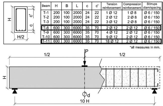
**FIGURE 2** Geometry of the beam specimens by Bosco and Debenardi<sup>29</sup>
