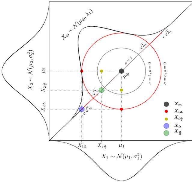
**FIGURE 1** Illustration of Eigen ECoV in standardized normal space with coordinates of realizations of input random vector.<sup>11</sup> ECoV, estimation of coefficient of variation
