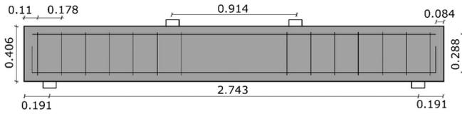
FIGURE 7 Geometry of the W1 beam of Anderson and Ramirez.<sup>30</sup> Note that the dimensions are in [m], but the original experiment was in imperial units
