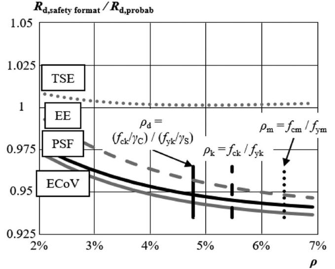
FIGURE 12 Variability of  $R_{d,safety\ format} / R_{d,probab}$  with  $\rho$
