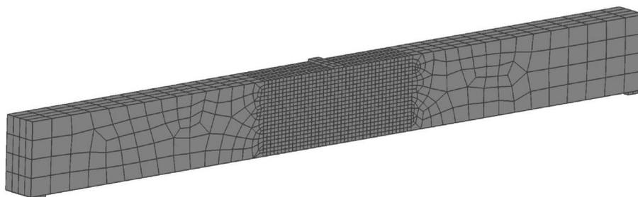
concrete. It should be noted that this assumption is not limiting since the bond failure can be captured quite well by the cracking of the finite elements next to the elements with the embedded reinforcement. The typical finite element mesh, shown in Figure 4, leads to an optimal number of finite elements (affecting computational costs) assuring the desired accuracy in the area of interest where the cracks develop.
