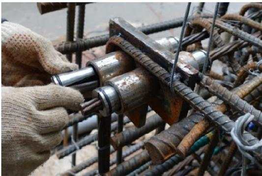
**Figure 65:** Wedges in the anchor during experiment.
