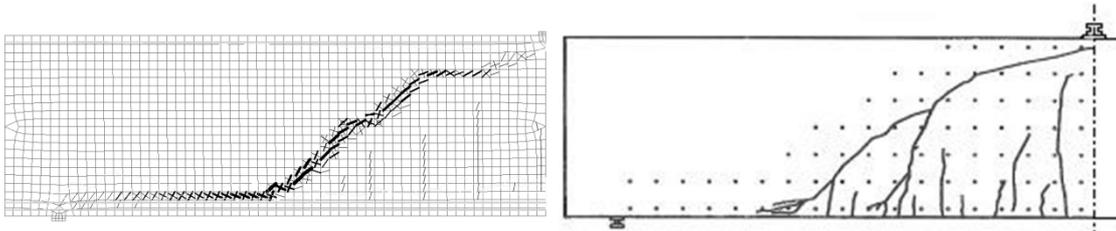
Fig. 3 Numerical and experimental crack pattern.
