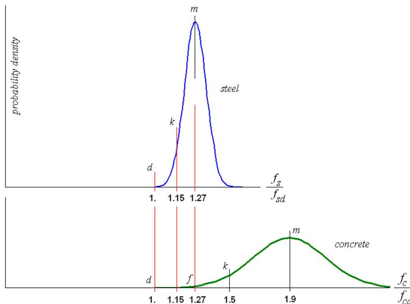
Fig. 1 Probabilistic definition of mean- $m$ , characteristic- $k$  and design- $d$  values for steel and concrete failure,  $f$ -reduced concrete strength.
