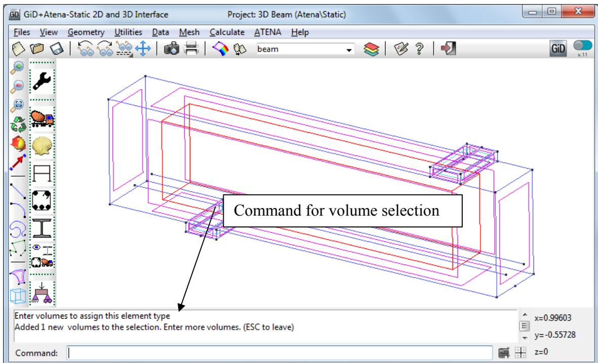
Figure 129: The selection of the beam volume
