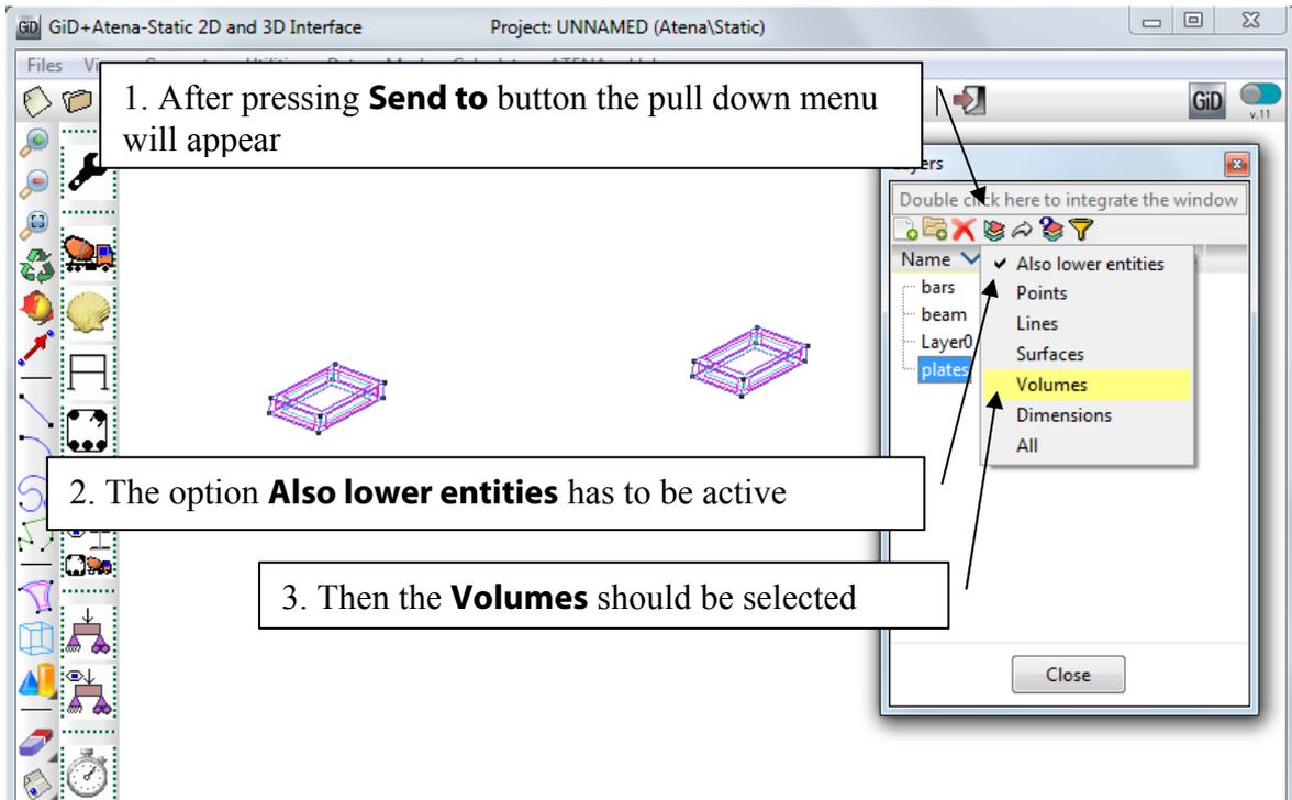
Figure 45: The definition of **Send to** command for the plates layer
