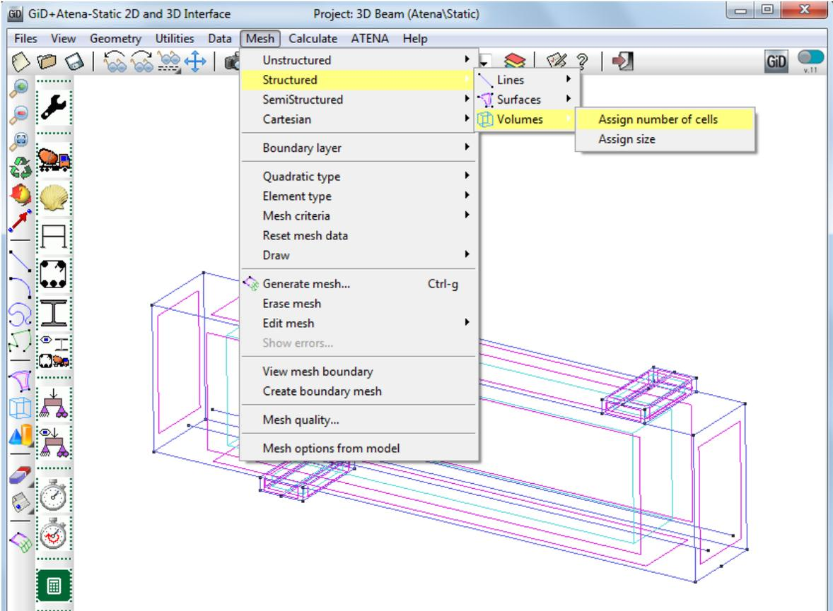
Figure 120: The Structured mesh command
