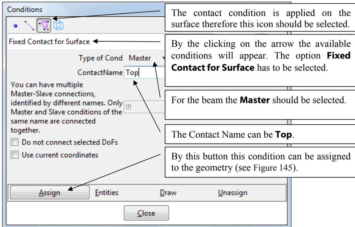
Figure 144: The master top beam contact condition
