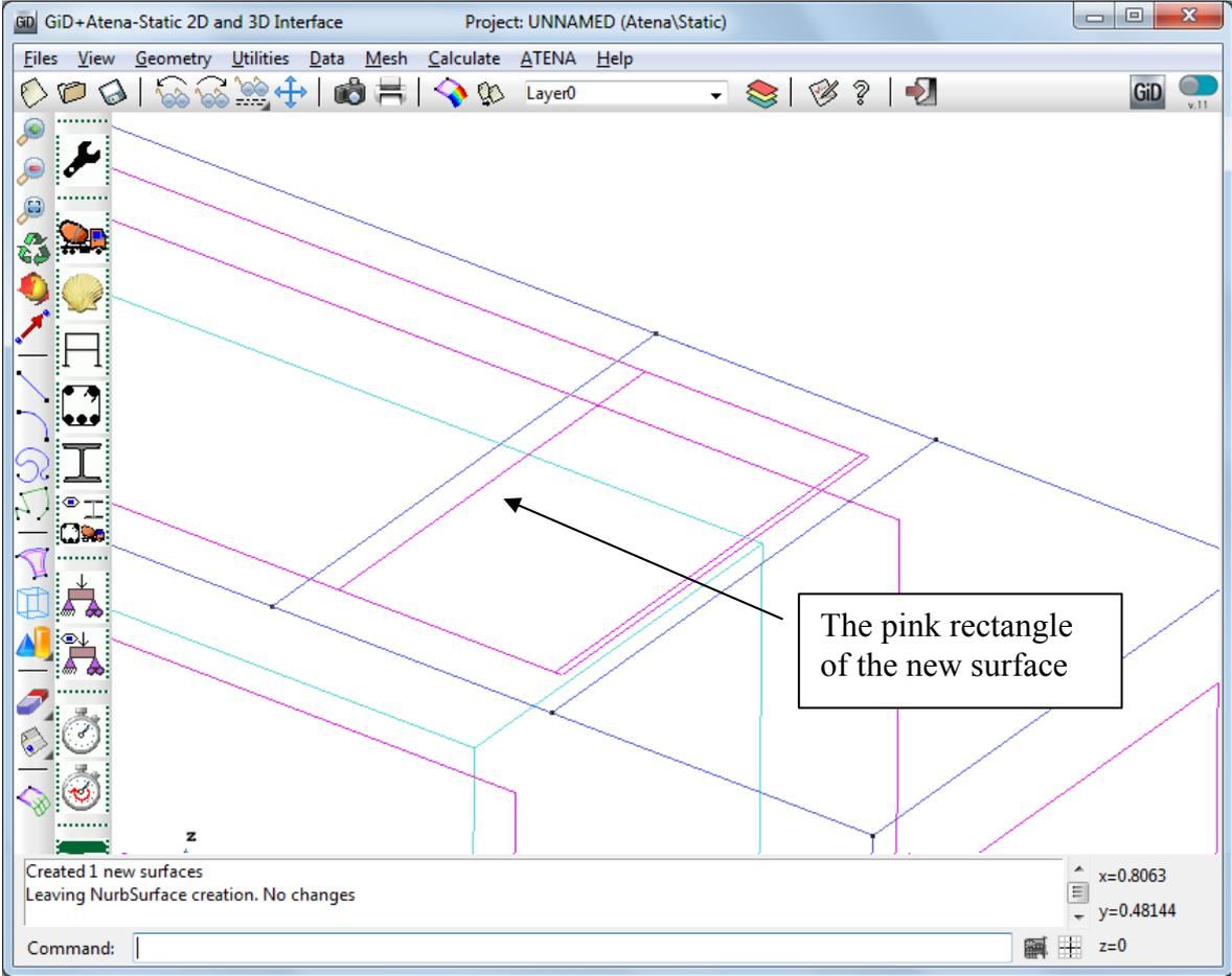
Figure 26: The surface created by automatic surface creation.
