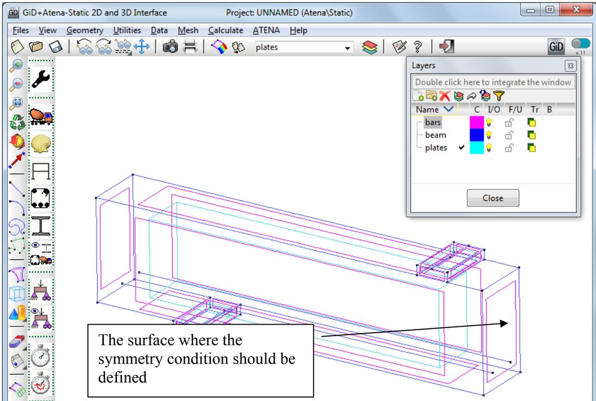
Figure 102: The surface for the symmetry condition
