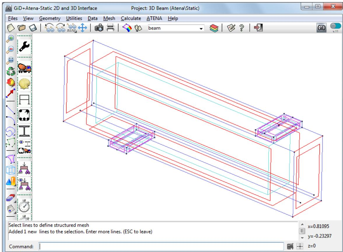
**Figure 127: The selection of the width lines**
