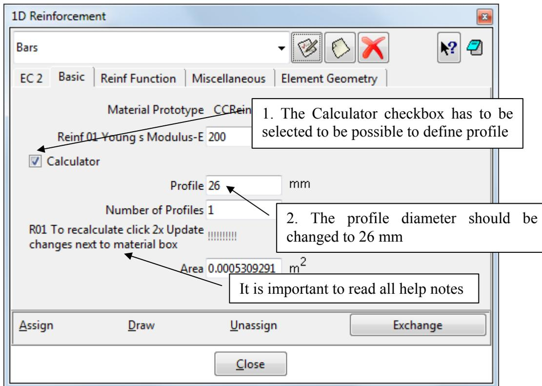
**Figure 76: The default Basic parameters of the reinforcement, the icon Update changes has to be dicked 2x to change parameters**
