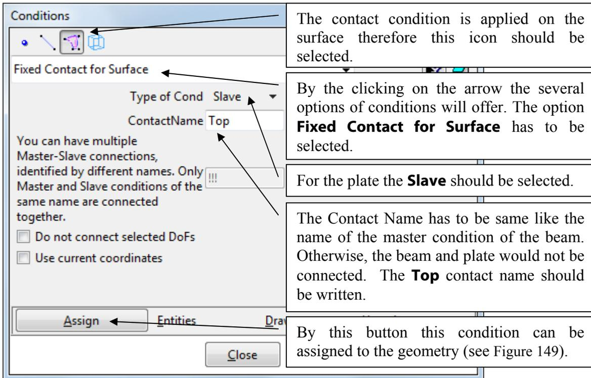
Figure 148: The slave top plate contact condition
