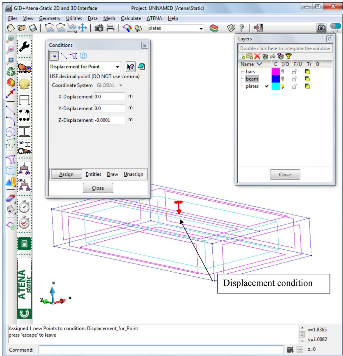
**Figure 101: The visual display of the displacement condition**
