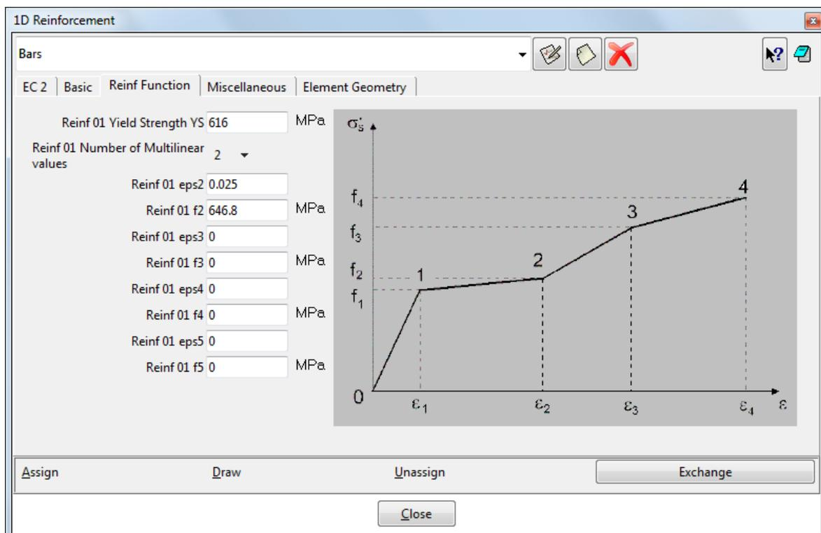
**Figure 77: The default Reinf Function parameters of the reinforcement**
