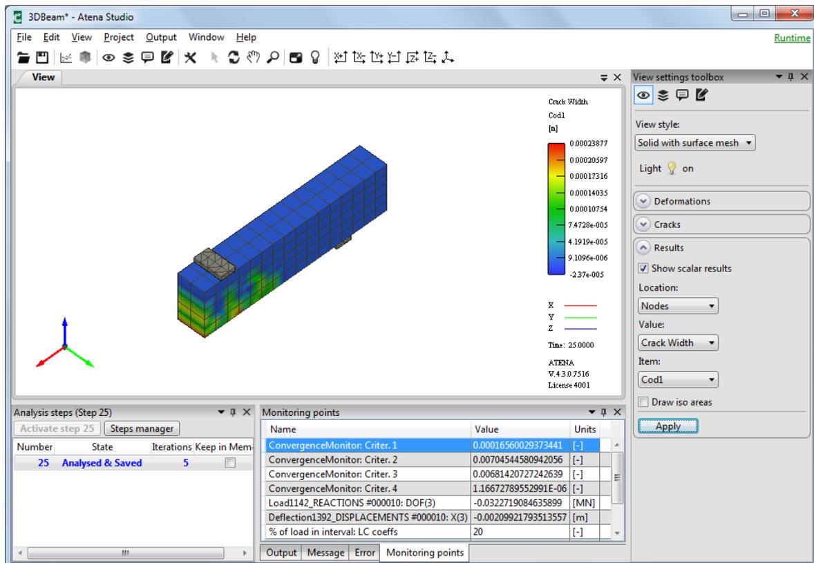
Figure 182: The crack width display of the 25<sup>th</sup> step
