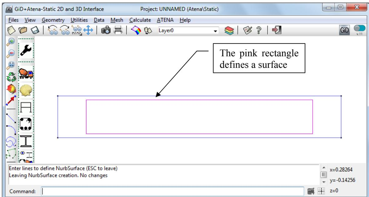
**Figure 11: The pink rectangle in the middle of blue lines defines the added surface.**
