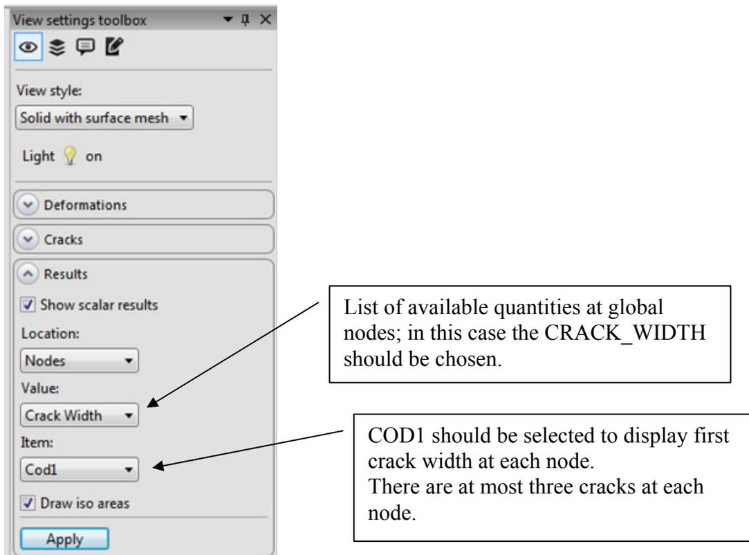
To update structure according to selected result press the button **Apply** (see Figure 161).
