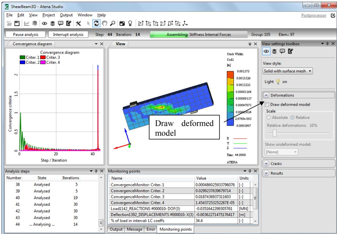
Figure 163: View settings toolbox with Deformations settings panel
