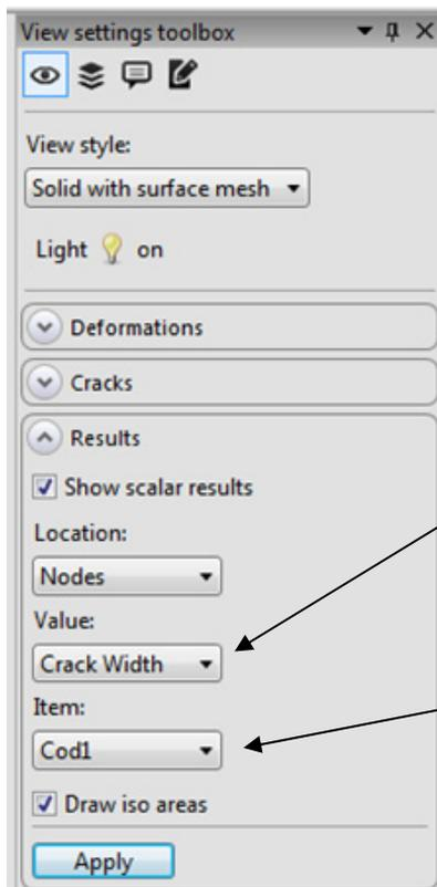
List of available quantities at global nodes; in this case the CRACK\_WIDTH should be chosen.
