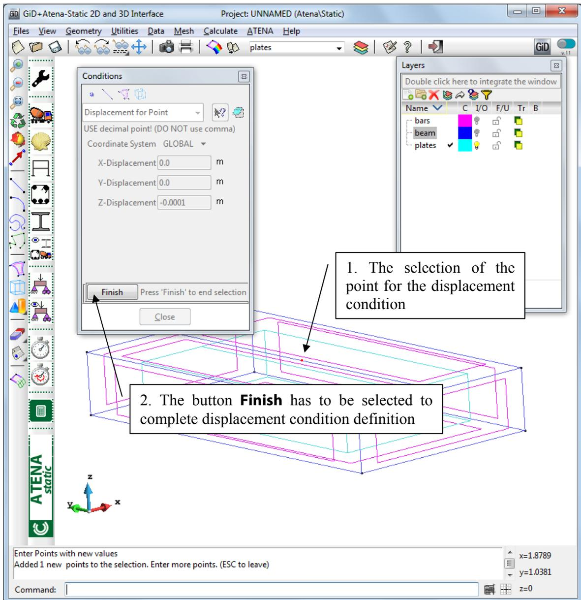
Figure 100: The selection of the point for the displacement condition
