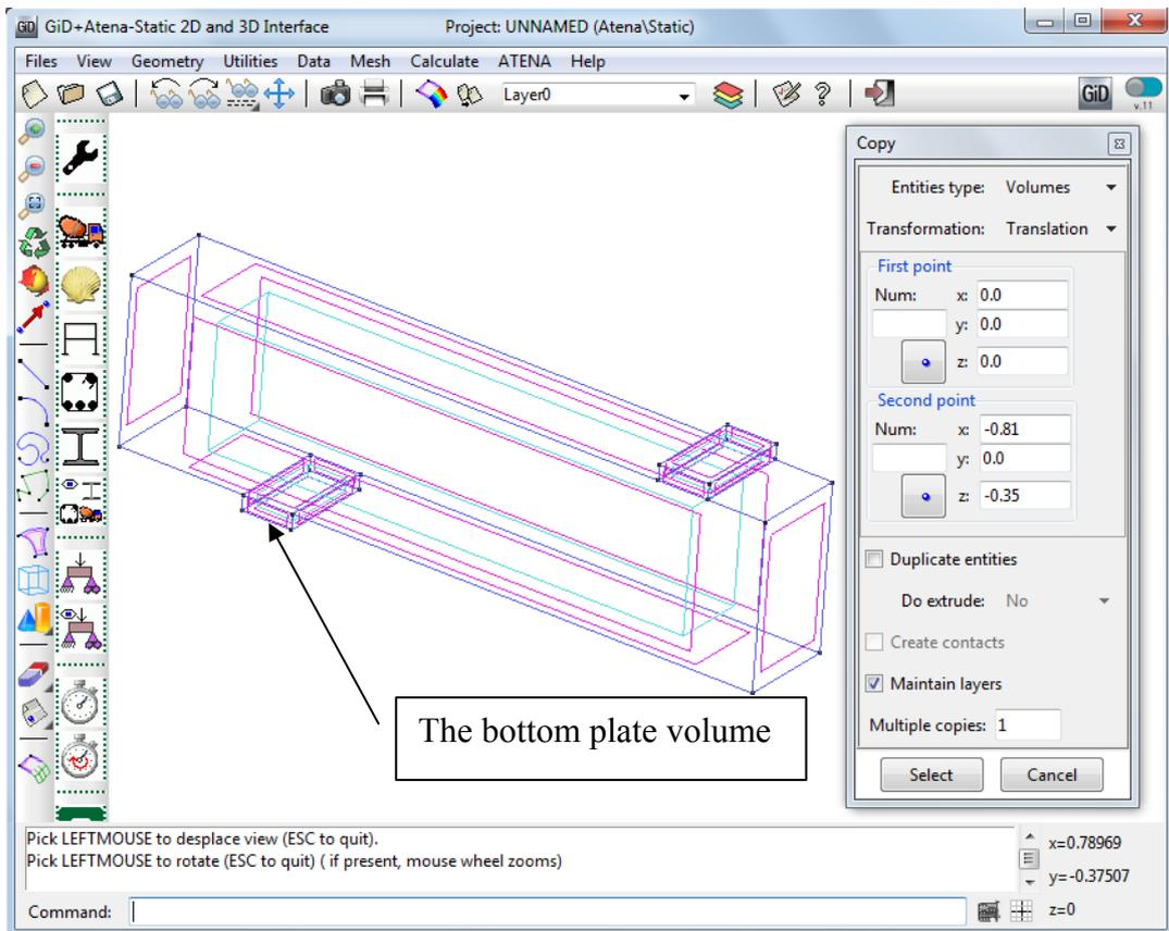
**Figure 32: The bottom and top plates**
