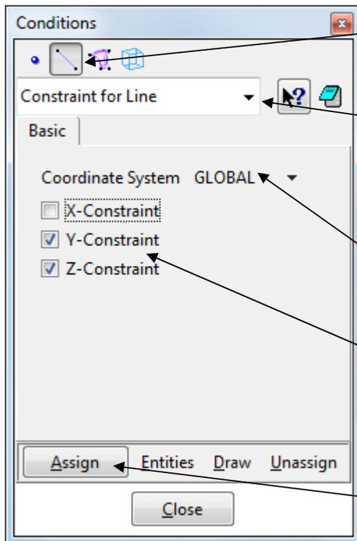
The support condition is to be applied on a line, therefore this icon should be selected.
