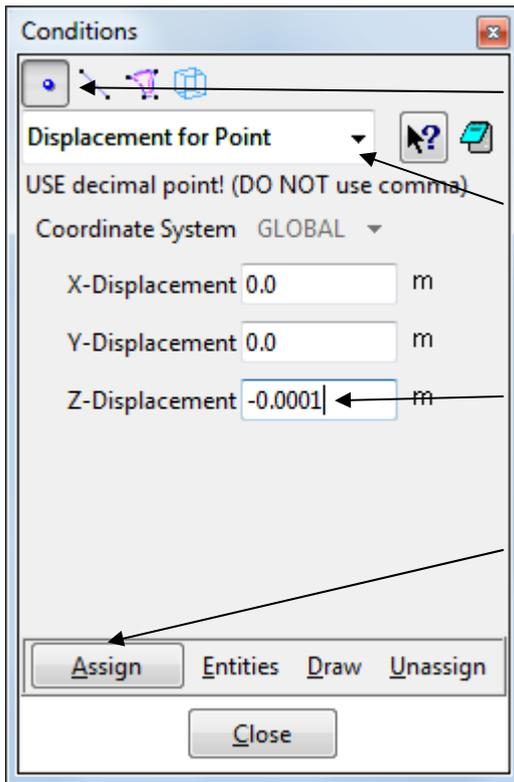
The displacement condition is applied on the point therefore this icon should be selected.
