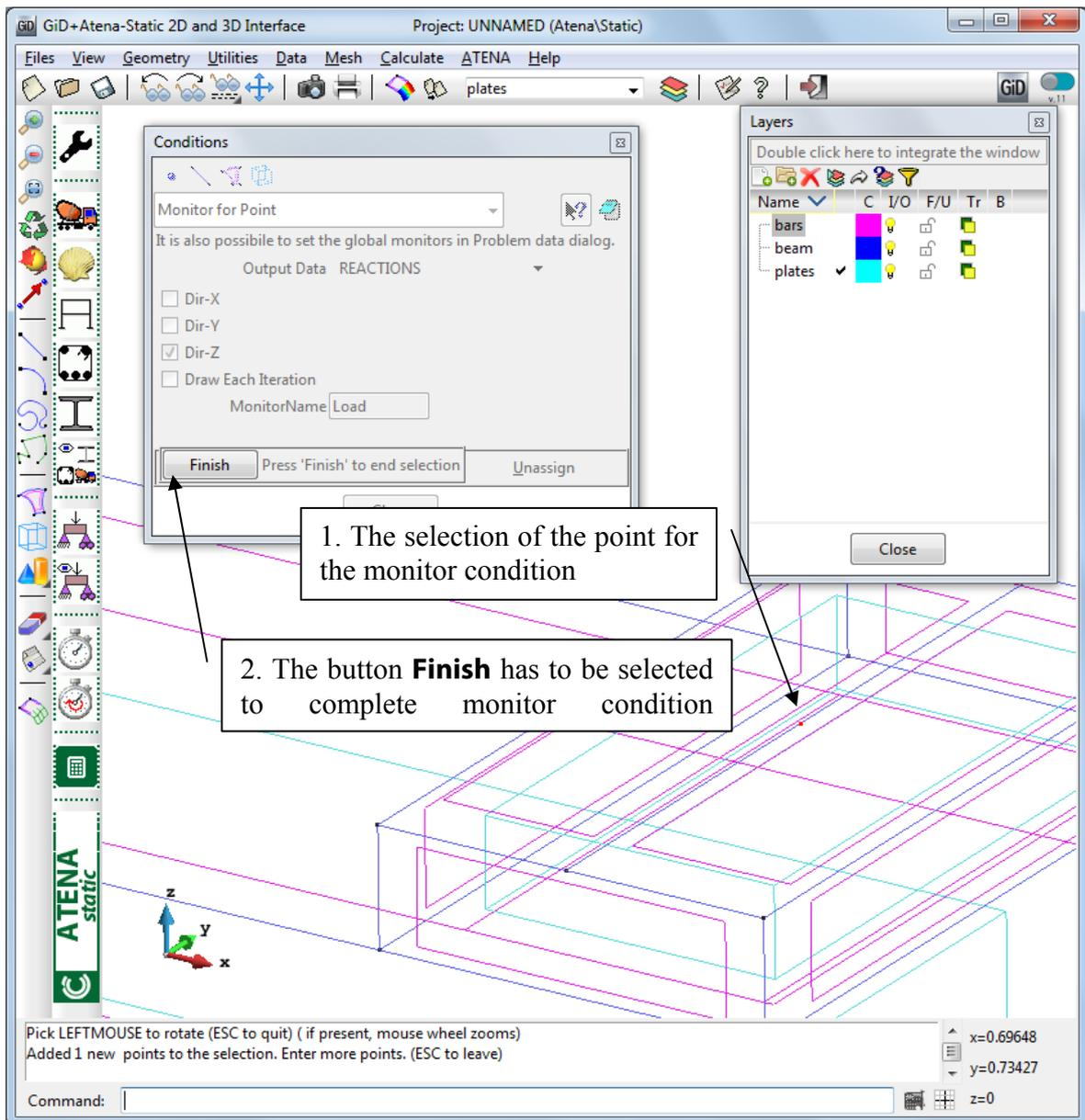
**Figure 107: The selection of the first monitoring point**
