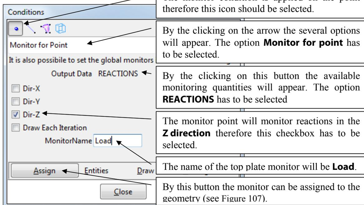
The screenshot shows the 'Conditions' dialog box with the 'Monitor for Point' option selected. The 'Output Data' is set to 'REACTIONS', and the 'Dir-Z' checkbox is checked. The 'MonitorName' field contains the text 'Load'. The 'Assign' button is highlighted. Callout boxes provide the following explanations:
