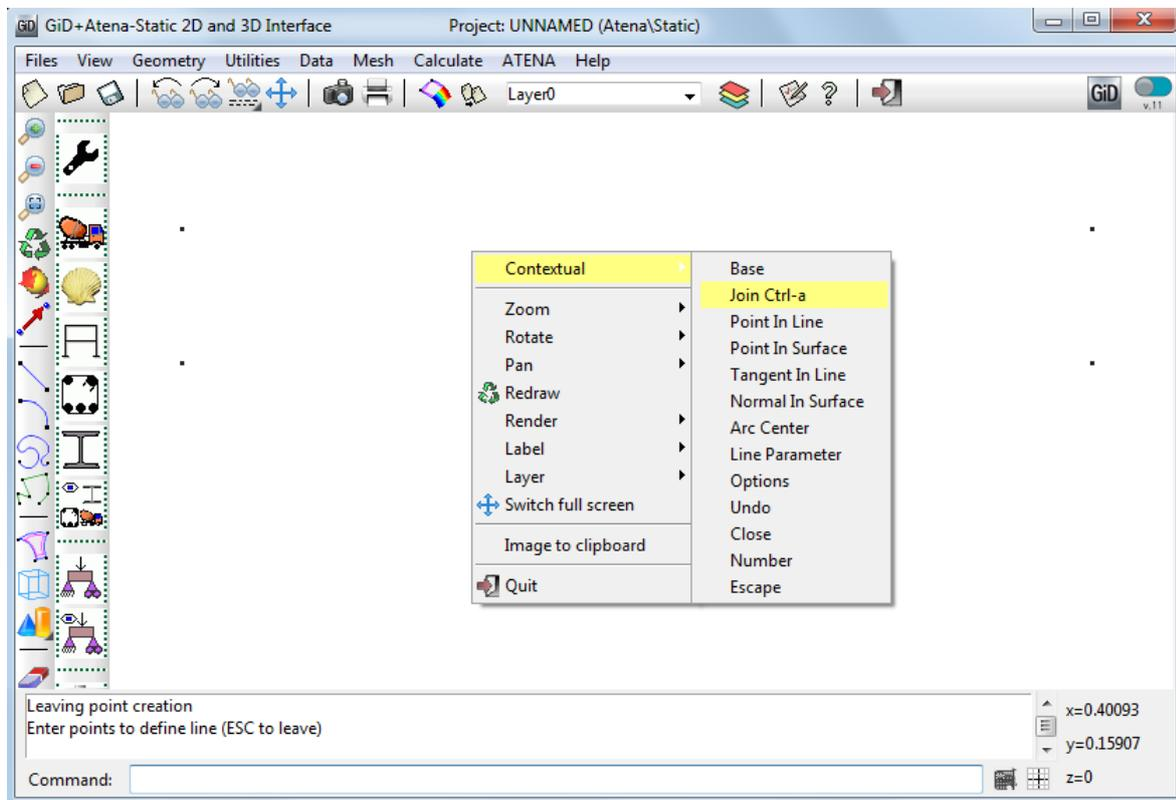
**Figure 9: The Join function in the Mouse menu.**
