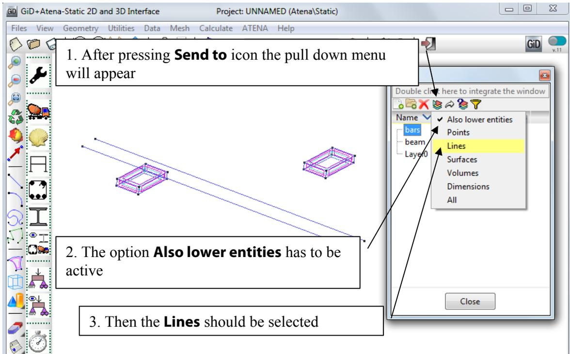
Figure 42: The definition of **Send to** command for the reinforcement layer
