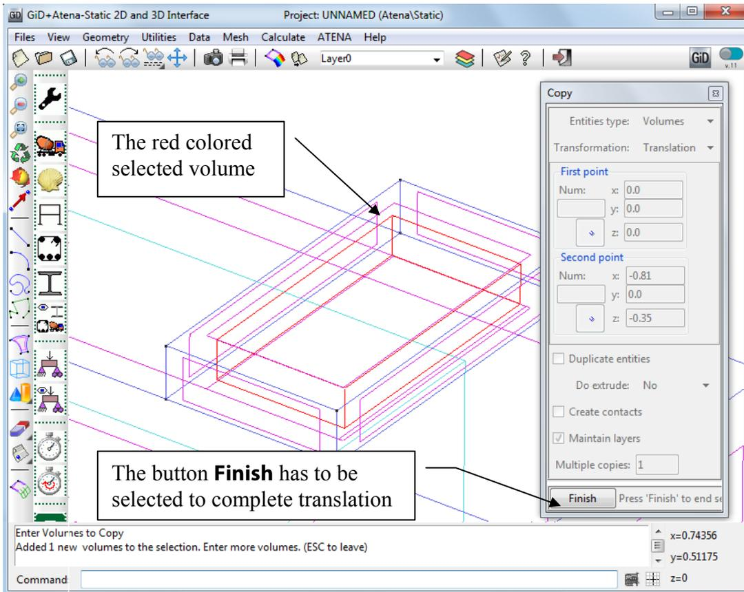
**Figure 31: The selection of the volume which should be copied**
