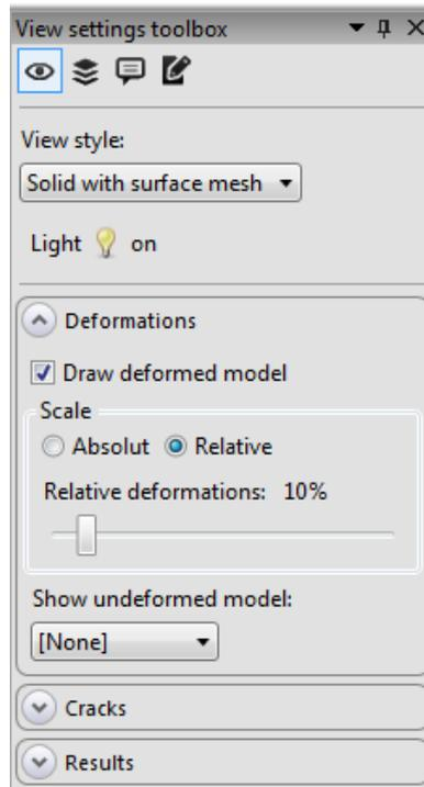
Figure 164: Deformed model settings
