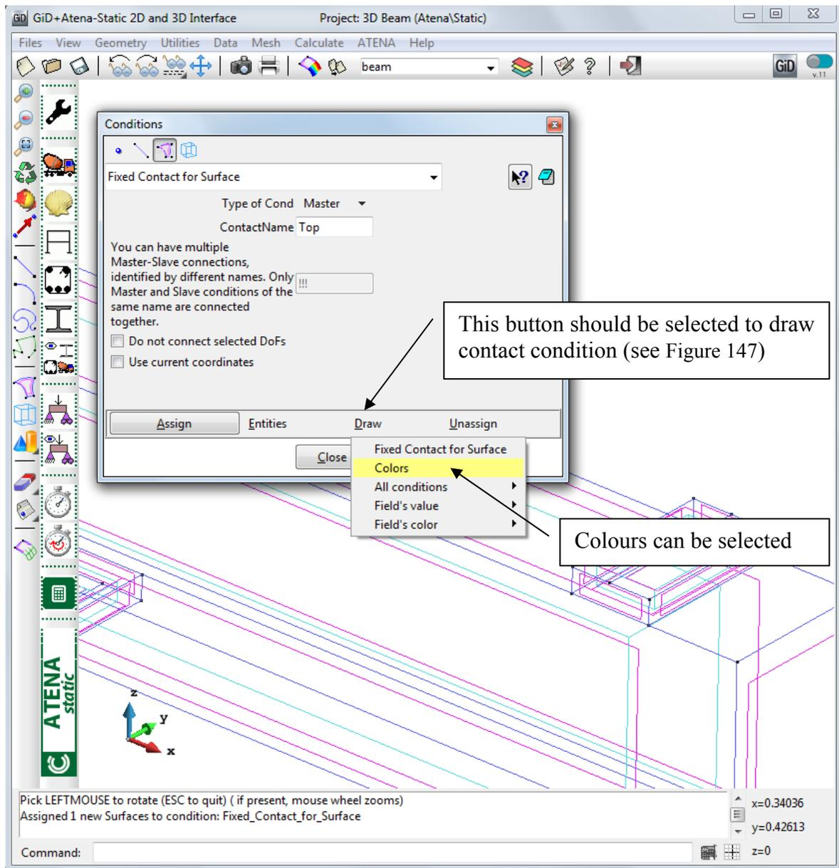
**Figure 146: The draw coloured contact condition command**
