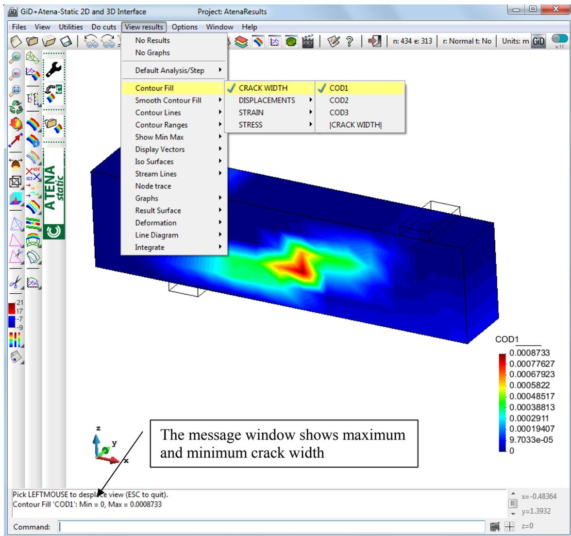
**Figure 174: The display of the crack width**
