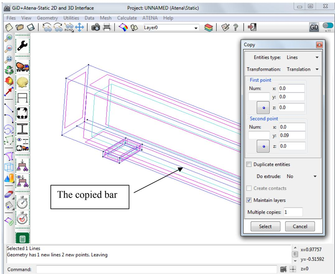
Figure 36: The first and second reinforcement bar
