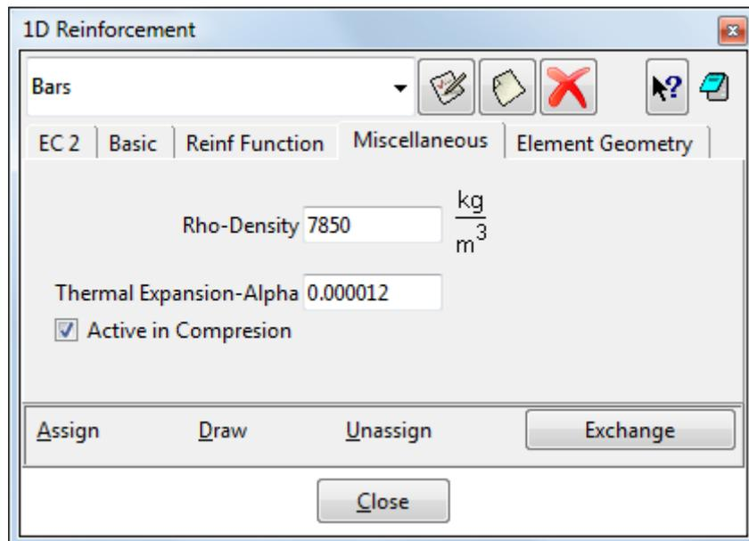
Figure 78: The default Miscellaneous parameters of the reinforcement
