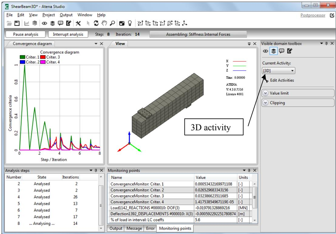
Figure 159: Visible domain toolbox with activity settings.
