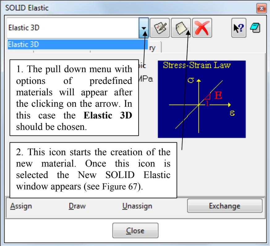
**Figure 66: Description of the new elastic material creation**
