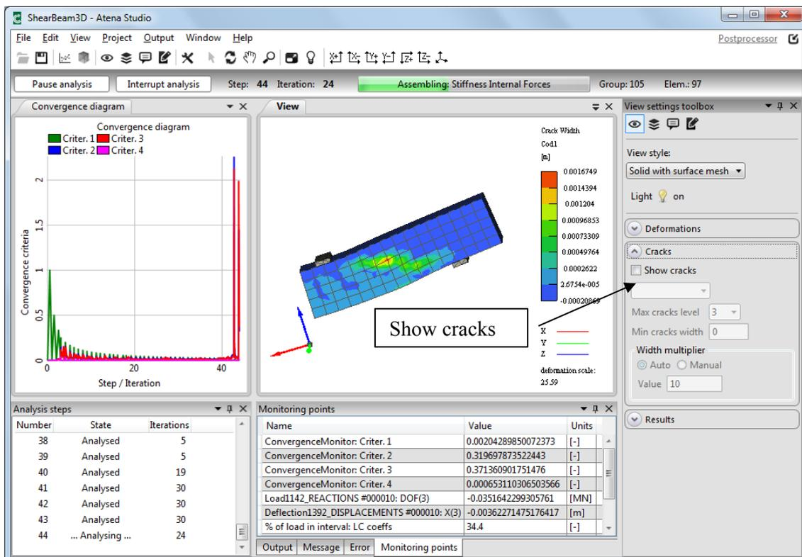
Figure 166: View settings toolbox with Cracks panel
