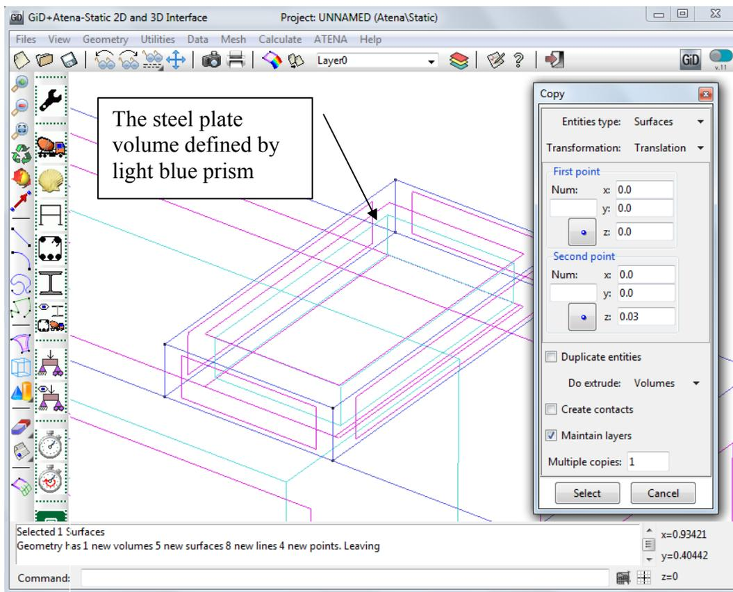
Figure 29: The volume of the top steel plate
