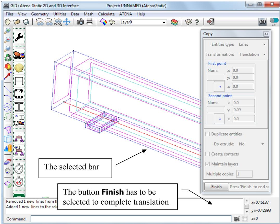
Figure 35: The selection of the first reinforcement bar which should be copied
