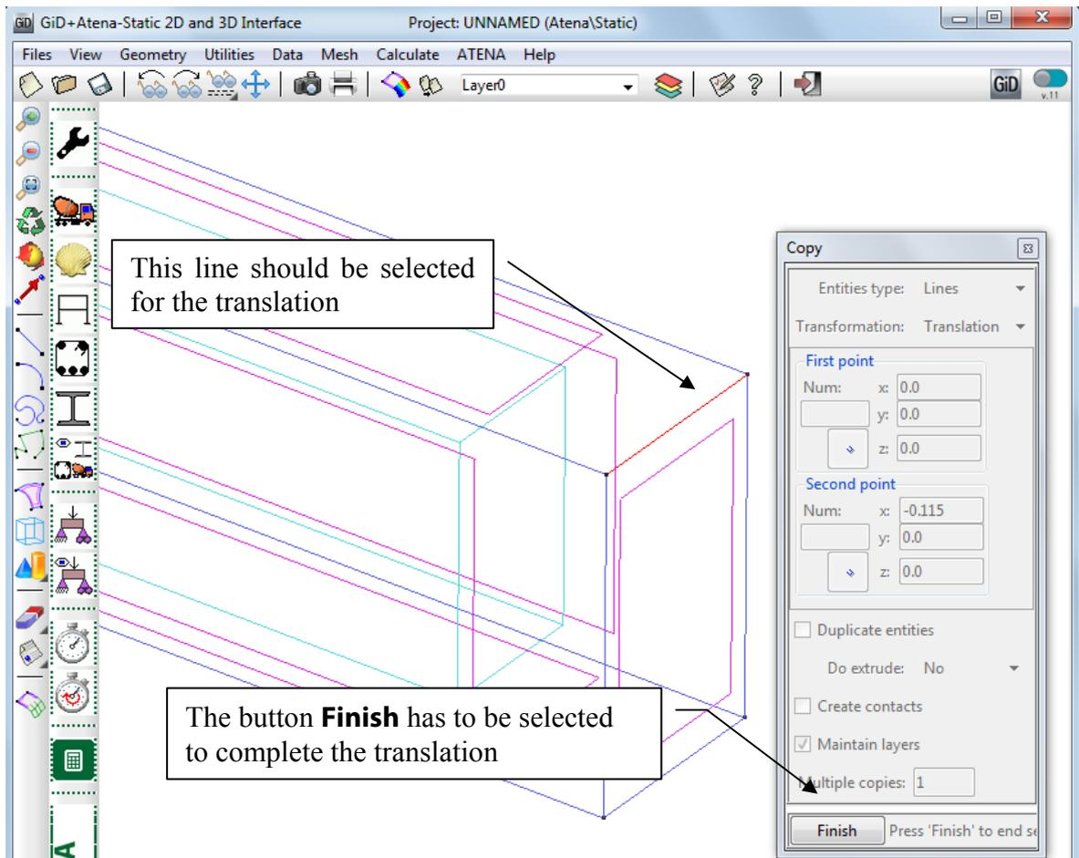
Figure 18: The selection of the line which should be copied
