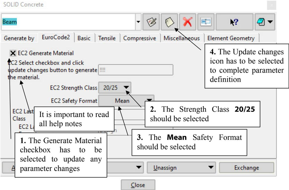
**Figure 57: The description of the class definition**
