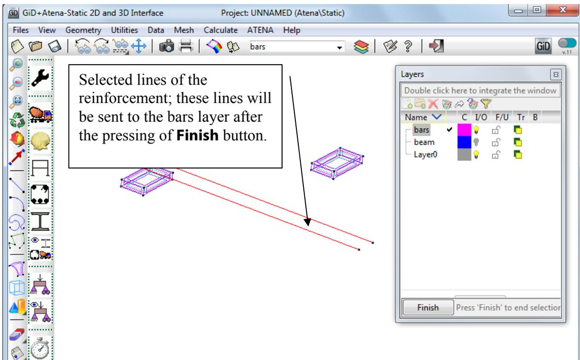
Figure 43: The selection of the lines, which should be sent to the bars layer
