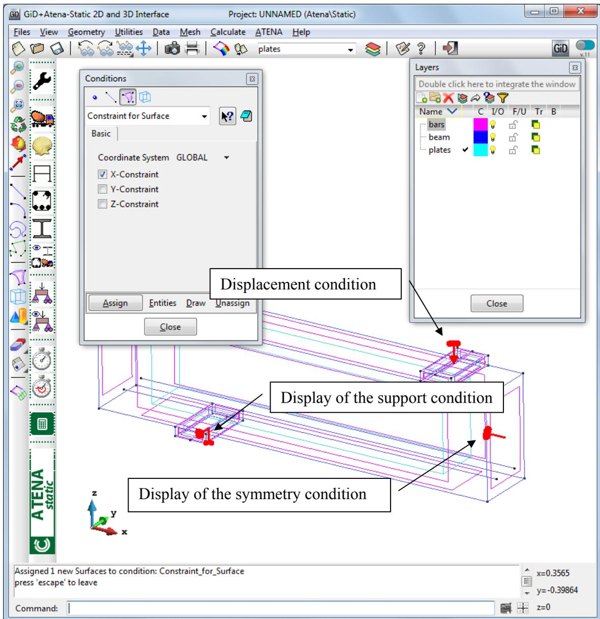
Figure 105: The visualization of the applied symmetry condition
