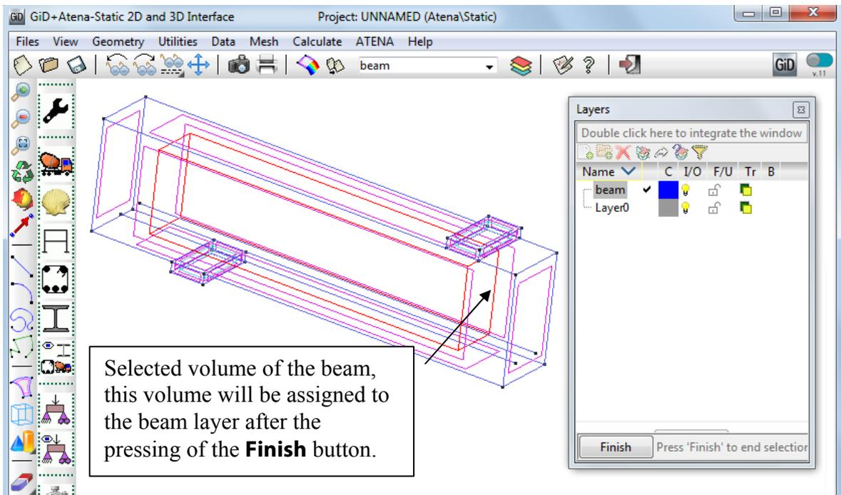
Figure 39: The selection of the volume, which should be sent to the beam layer
