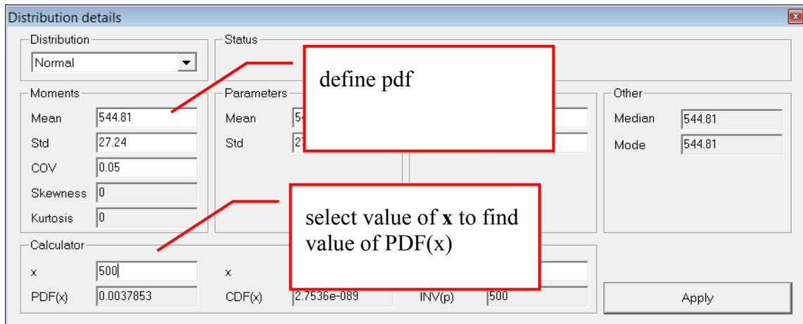
Figure 66 Finding particular value of a PDF
