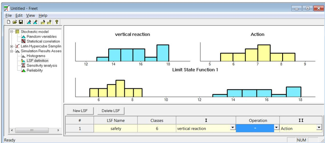
Figure 85 Definition of a new limit state function
