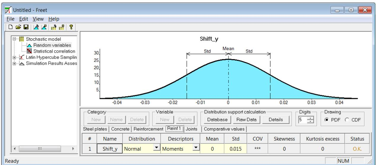
Figure 52 FReET – vertical coordinate of reinforcing bar is randomized
