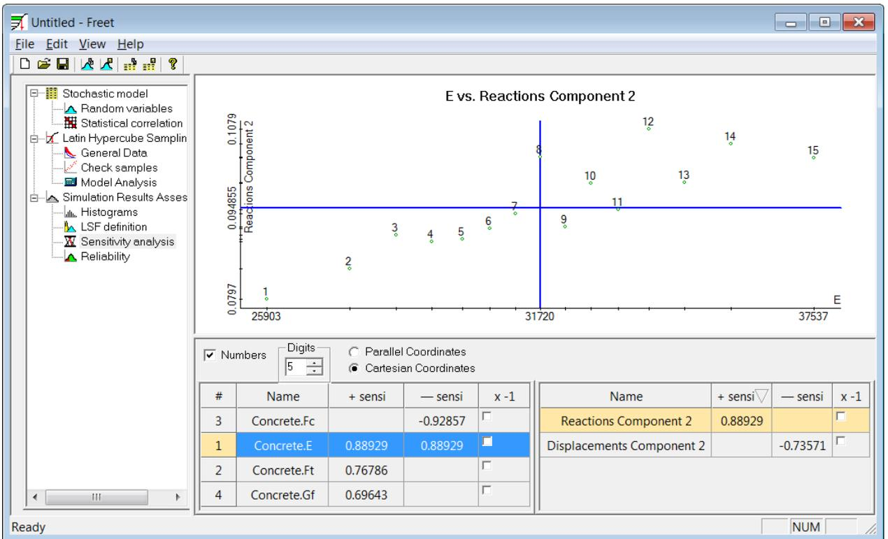
**Figure 30 FREET – Sensitivity analysis of Reaction component 2 on Young’s modulus E (Cartesian coordinates)**
