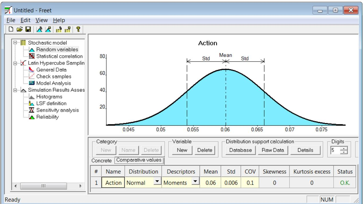
Figure 31 FREET – definition of a new comparative value named “Action”
