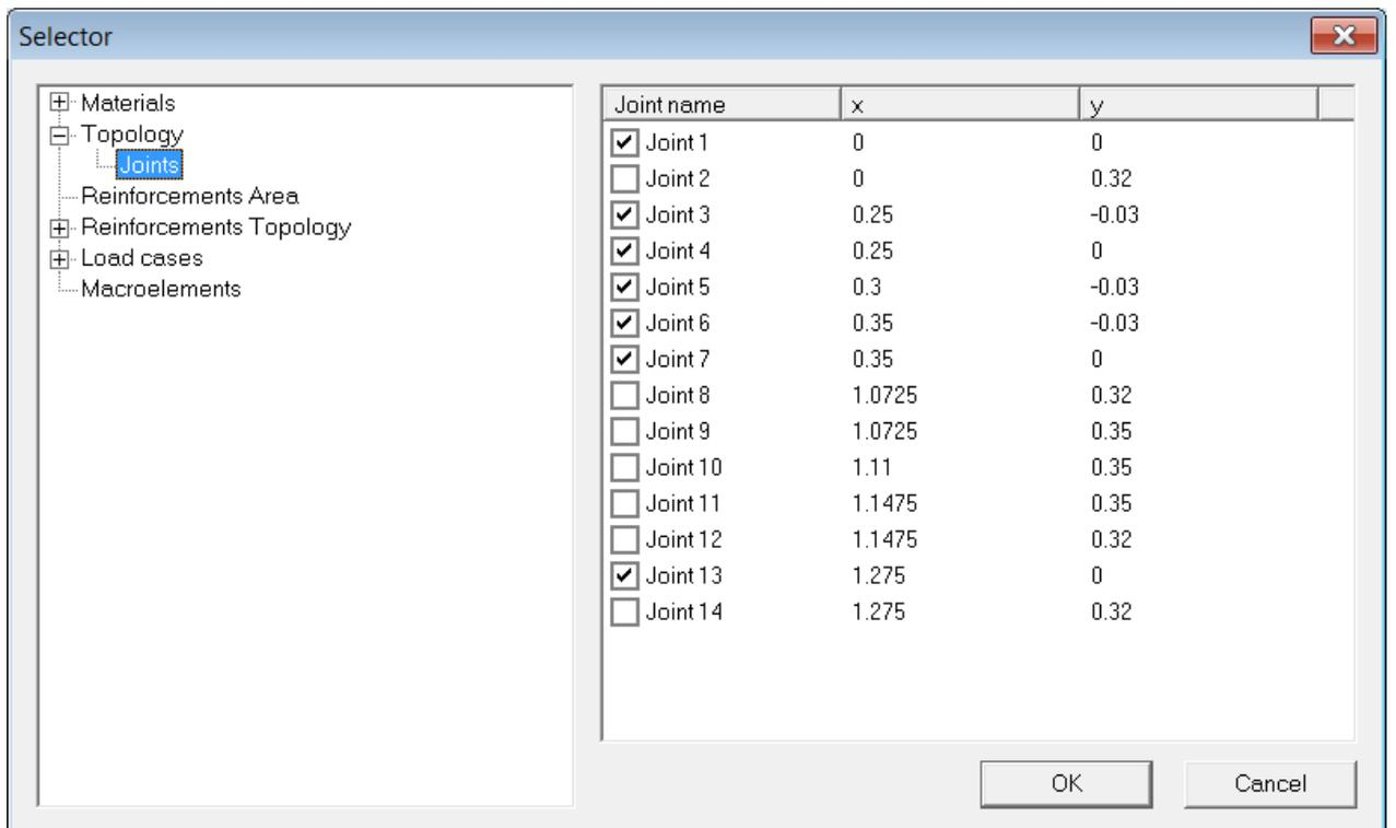
Figure 49 Selector – selection of joints located at the bottom of the beam (+ bottom loading plate)
