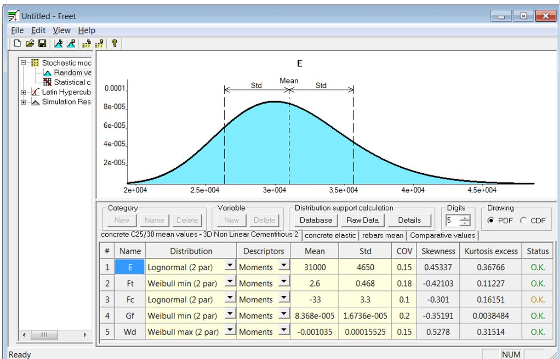
Figure 80 Probabilistic distribution for concrete C25/30 parameters
