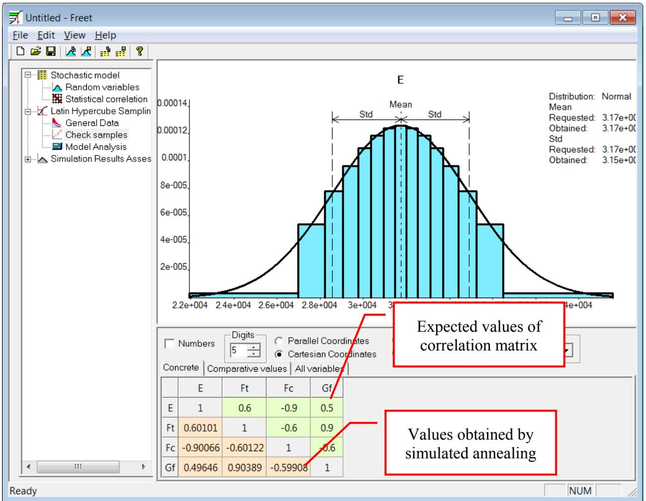
Figure 17 Freet – generated parameters
