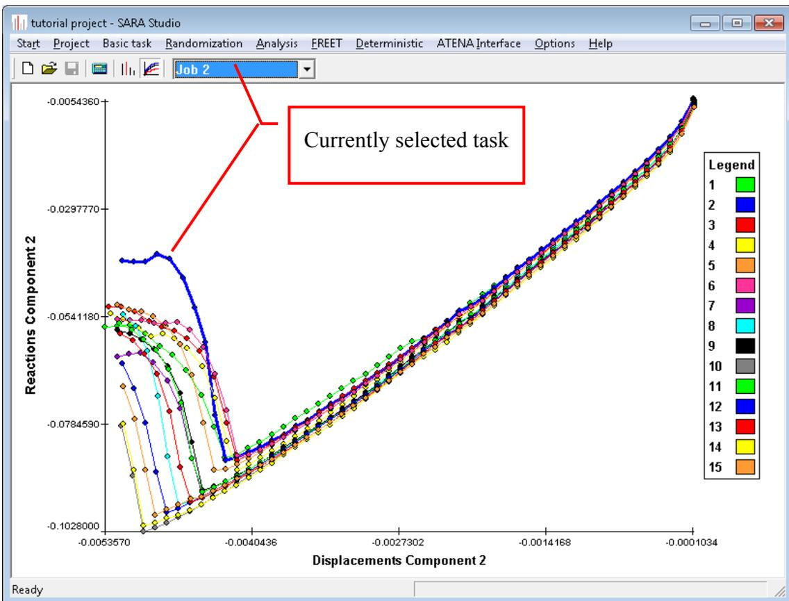
Figure 26 Finished analysis – Line chart view
