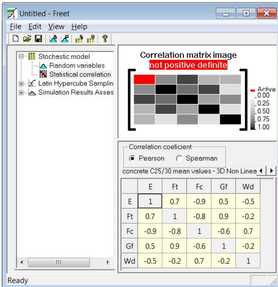
Figure 82 Definition of correlation matrix for material C25/30.
