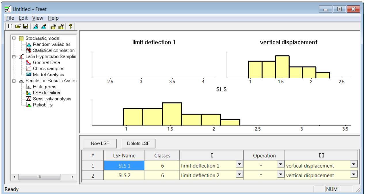
Figure 91 Definition of limit state functions.
