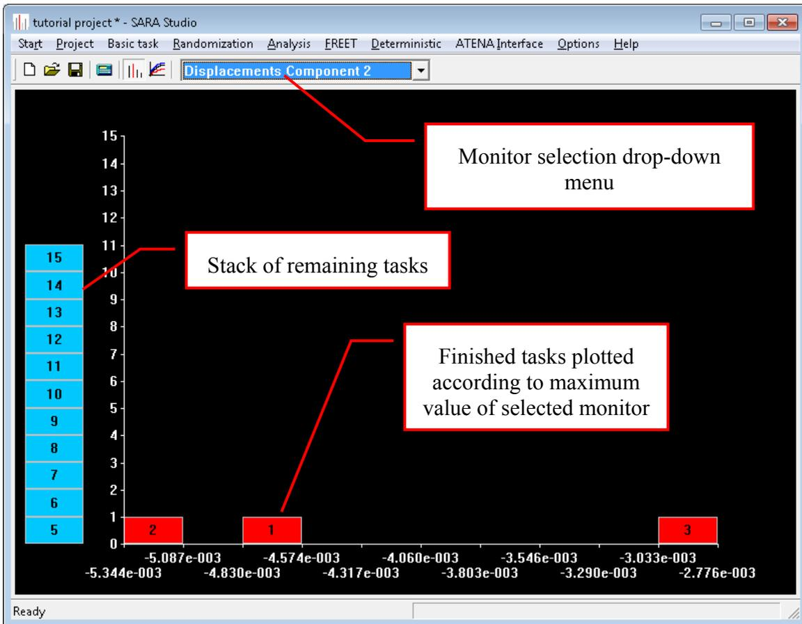
Figure 22 Simulation progress – three finished task and 15 remaining
