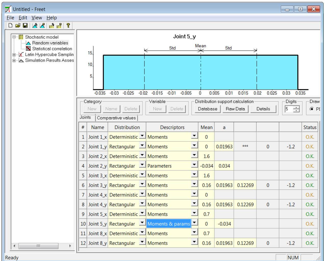
Figure 75 Probabilistic distribution of joints
