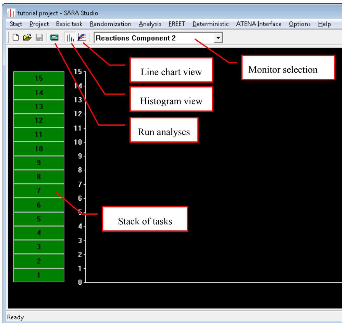
Figure 18 SARA Studio – stack of inputs ready to be computed
