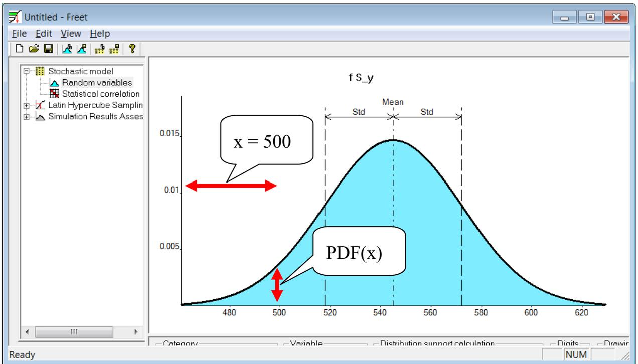
Figure 67 Finding particular value of a PDF
