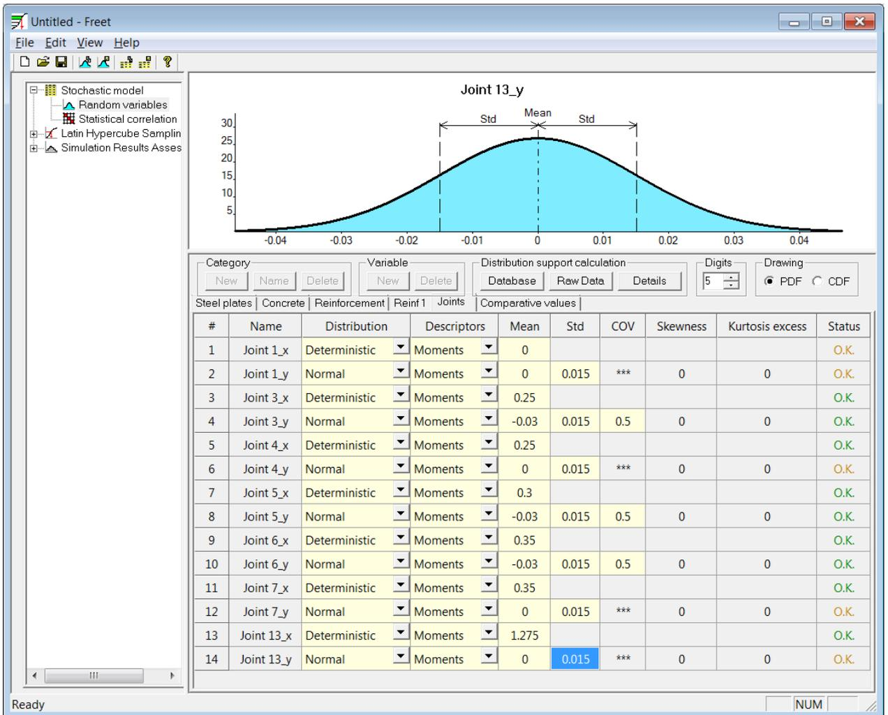
Figure 51 FReET – vertical coordinate of all selected joints is randomized
