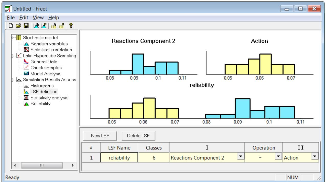
Figure 32 FREET – definition of a new limit state function
