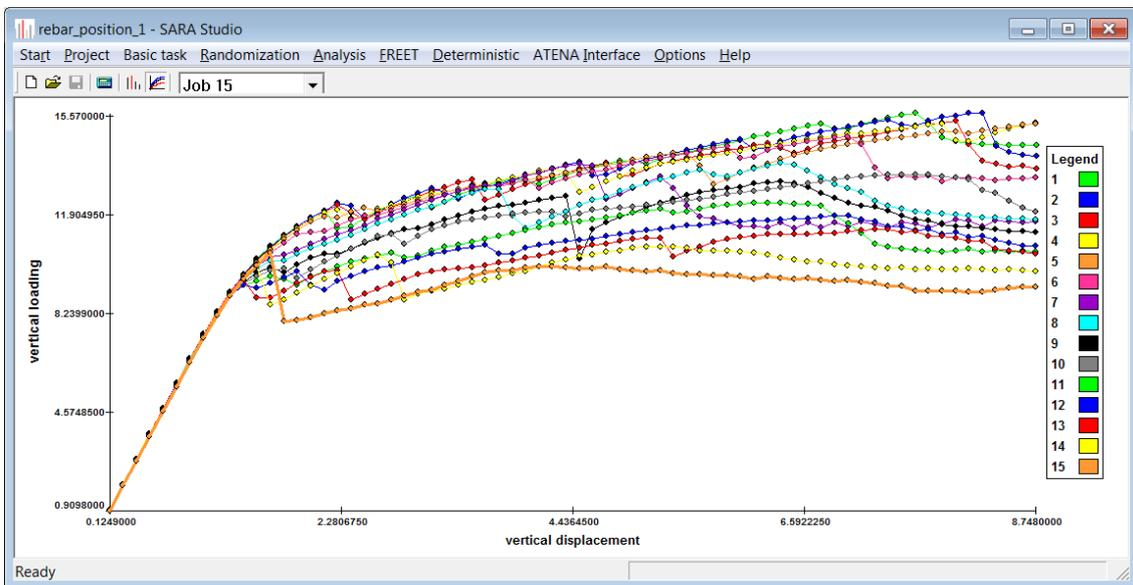
Figure 77 LD diagrams of 15 variants (5Ø8)
