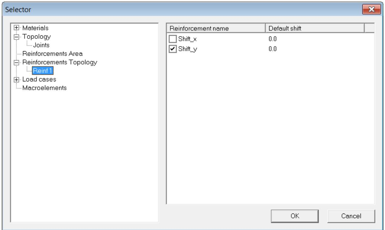
Figure 50 Selector – vertical movement of reinforcing bars is chosen for randomization
