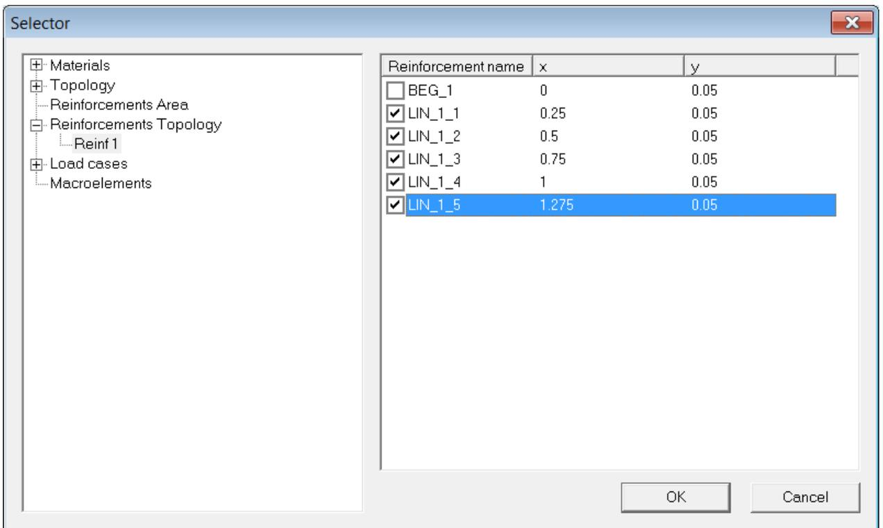
Figure 47 Selector – Reinforcement Topology – Reinf1 is expanded to display all points defining reinforcing bar
