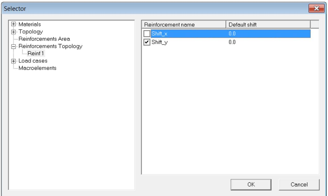
Figure 44 Selector – Reinforcement Topology – Reinf1 is expanded to display vertical and horizontal component of shift.
