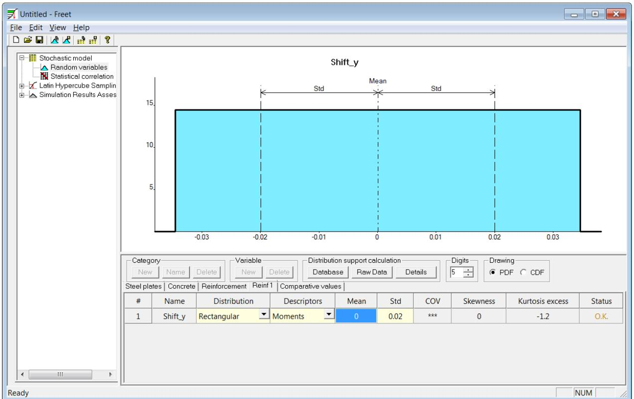
**Figure 45 Freet – randomization of rebar position**
