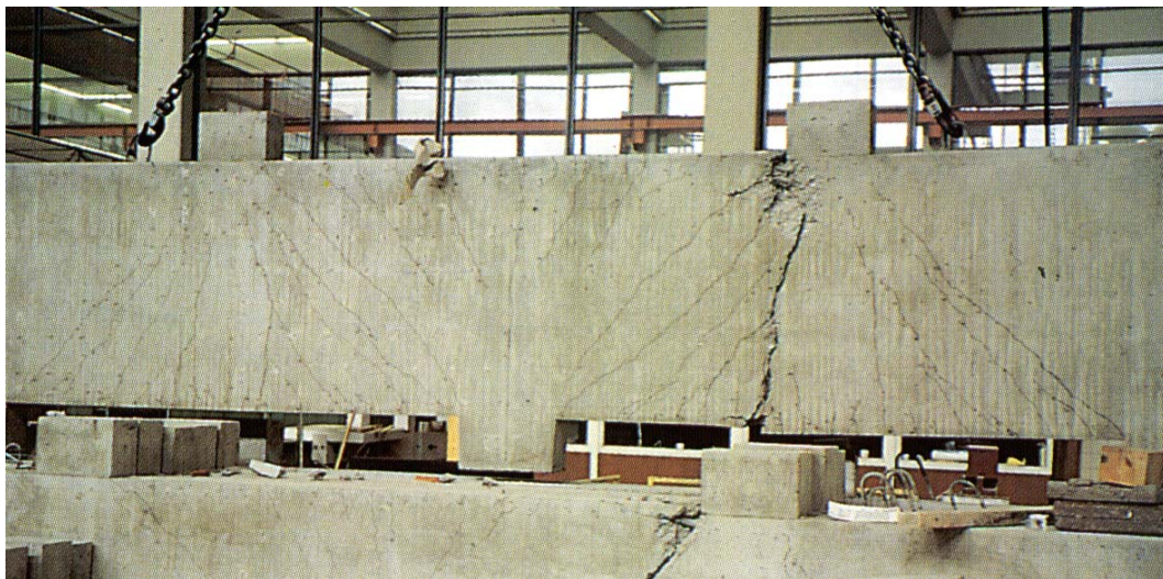
Figure 5: Shear wall tested in the laboratory, Asin (1999)
