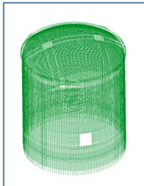
Model of prestressing cables in a nuclear containment vessel.
