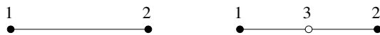
Figure 1: Node numbering of an edge element (linear element – left, quadratic and quadratic bubble element – right). Symbols: full circle – corner node, empty circle – midedge node
