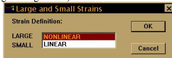
Fig. 9 Large and small strain option.
